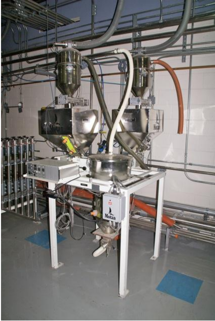
Two (2) Motan Compound blender with control unit (two 600 lb drying bins not shown)
