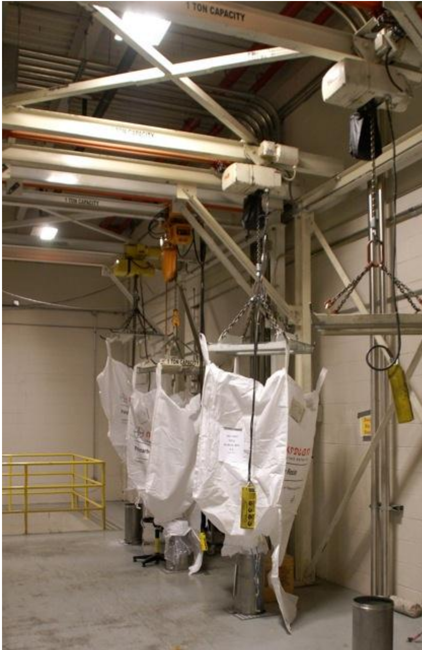
Four Yale (1) one ton hoist/trolleys for hanging super sacks
