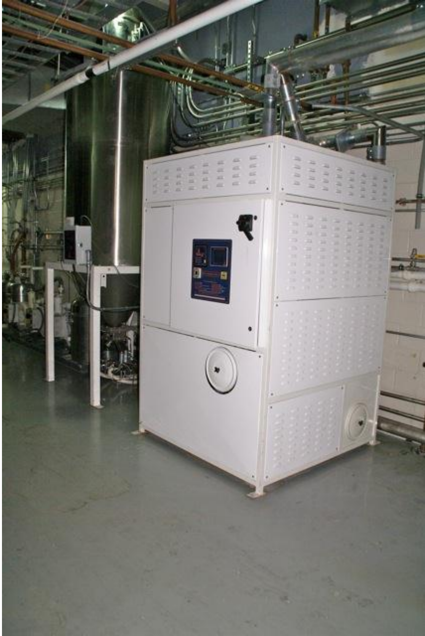
Motan 2500 lb drying bin with Motan diagnostic dryer Model # MDD 800 (480/3/60)
