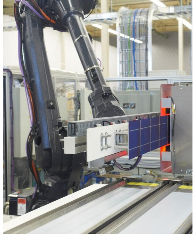
String inspection at the Photowatt Ontario facility in Cambridge, ON.
