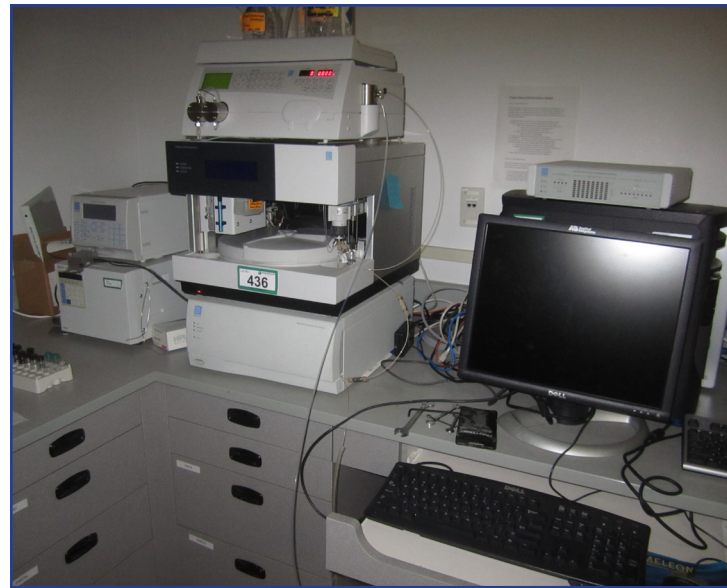
Thermo Finnigan AQA Mass Spectrometer Waters Micromass: Mass Spec System with HPLC and liquid handling components; Includes (1) Waters Micromass Zqmass Spec with EXCI multi-mode ionization enabler (3) Waters 515 HPLC pump (1) Waters 2487 Dual Absorbance Detector (1) Waters Column Fluidics Organizer (1) 2525 Binary Gradient module (1) Waters Pump control module II (1) Waters 2767 Sample Manger (1) IBM thinkcenter computer and monitor
