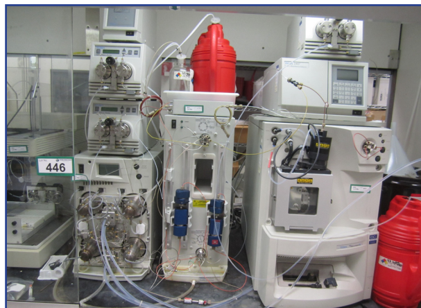
Waters/Micromass Quattro Premier XE: Mass Spectrometer with UPLC System; Includes [Waters Acquity Ultra Performance LC System with Sample manager, Sample Organizer, and Binary Solvent Manager] [Also includes Lenovo Think Center Computer and Monitor, accessories, and cart]
