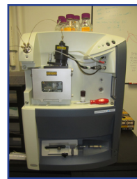
Thermo Finnigan AQA Mass Spectrometer Waters Micromass: Mass Spec System with HPLC and liquid handling components; Includes (1) Waters Micromass Zqmass Spec with EXCI multi-mode ionization enabler (3) Waters 515 HPLC pump (1) Waters 2487 Dual Absorbance Detector (1) Waters Column Fluidics Organizer (1) 2525 Binary Gradient module (1) Waters Pump control module II (1) Waters 2767 Sample Manger (1) IBM thinkcenter computer and monitor
