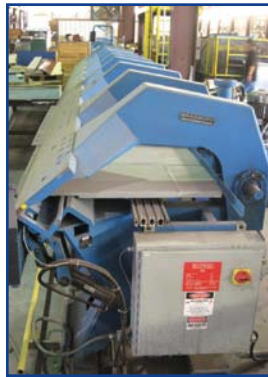
Bradbury Model Folder 14-33' x 14 Gage CNC Hydraulic Long Folder Panel Former
