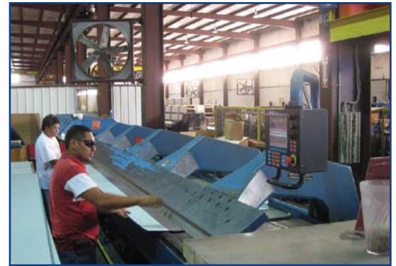
Bradbury Model Folder 14-33' x 14 Gage CNC Hydraulic Long Folder Panel Former
