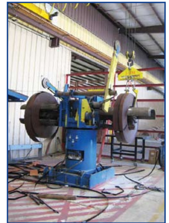
Geka Model Hydracrop 110-SD CNC Hydraulic Ironworker, (2006), 6.5" x 6.5" x 1.5" Angle Shear, 24" x 5/8" Channel, 2" Dia. Tube, 2" Dia. Pipe, with Fagor CNC Controls
