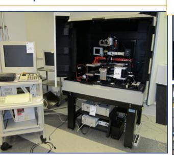
Hypervision Visionary 2000 Light Emission Microscope With Karl Suss PM-8, Mitutoyo Objectives: (1) M Plan 50 NIR, M Plan NIR 20, M Plan NIR 5, Light Source, 2 chucks. Computer and Monitor, TMC Micro-G Vibration Table.
