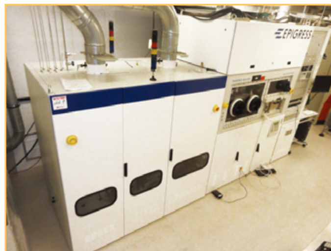
AXITRON EPIGRESS TYPE VP 2400 HW, GAS FOIL ROTATION PLANETARY REACTOR
