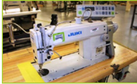
JUKI DLN-5410N-7 WB SINGLE NEEDLE LOCKSTITCH
