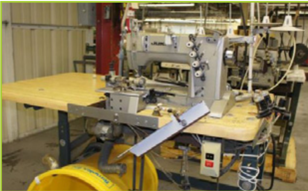
JUKI MFB-2600 CLASS HHM DOUBLE NEEDLE CHAINSTITCH WITH PULLER
