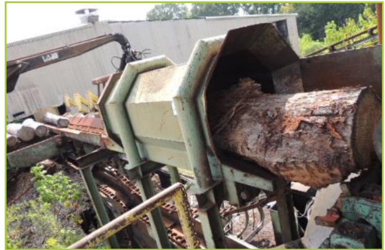
60' OUTFEED LOG TROUGH CONVEYOR WITH S DRIVE CONSTRUCTION AND H-132 LUG CHAIN
