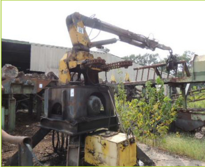
HUSKY STATIONARY KNUCKLEBOOM LOADER WITH MOTOR AND HYDRAULIC PACK
