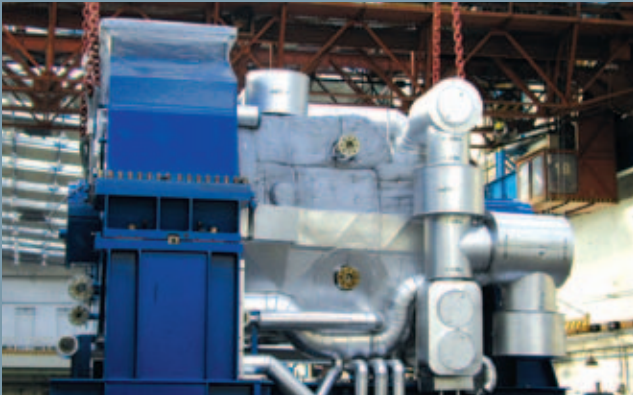
SST-400, Burnaby, BC, Canada; 25 MW. The condensing extraction turbine powers an incineration plant.
