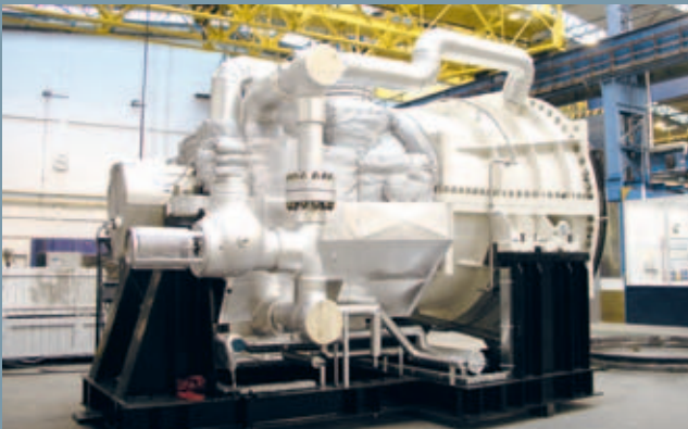
SST-400, Kayseri, Turkey; 35.5 MW. Condensing turbine for a combined cycle plant.
