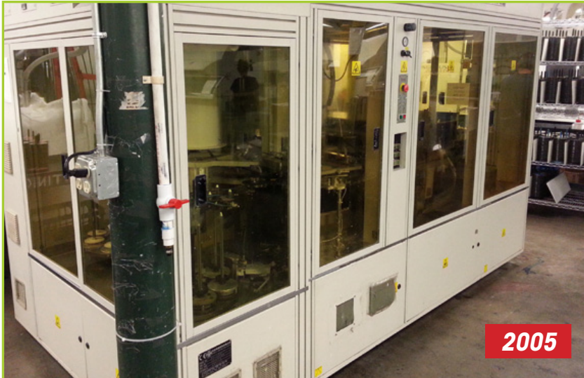
HANKY HS 420-P HANKY OFFSET PRINTER FOR CD AND DVD, MODEL HS-420P, YEAR 2005
