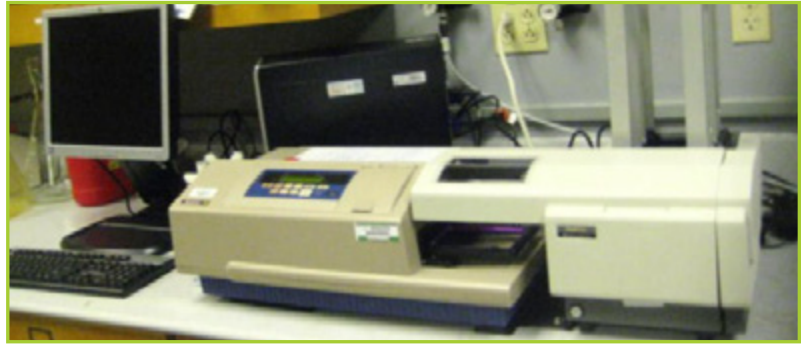
MOLECULAR DEVICES M5 SPECTRA MAX MULTI FUNCTIONAL MICRO PLATE READER
