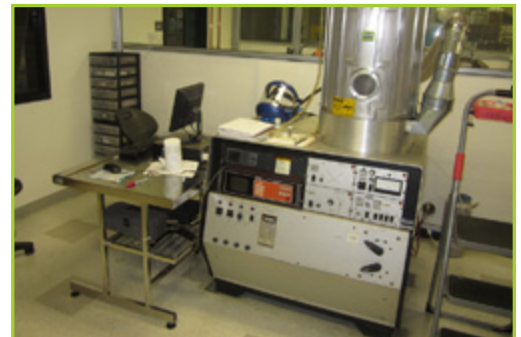
CHA INDUSTRIES CHA 600 THERMAL EVAPORATOR SYSTEM
