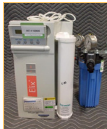
MILLIPORE ELIX 3UV WATER PURIFICATION SYSTEM
