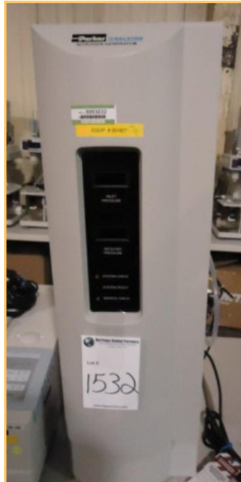
PARKER BALSTON HPN2-1100 NITROGEN GENERATOR
