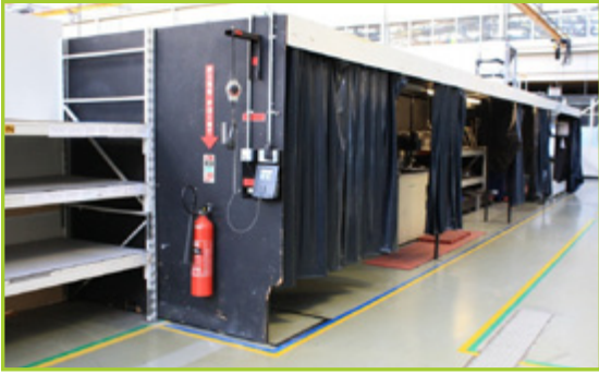
MULTIPLE BLACKOUT INSPECTION BOOTHS
