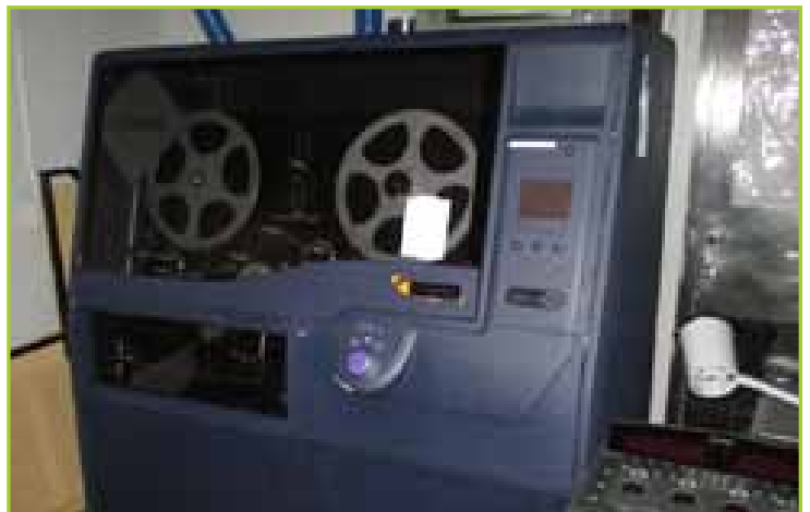
CINTEL PROFESSIONAL C-REALITY COLOR VECTOR IMAGING PROCESSOR
