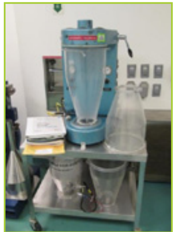
NIRO-AEROMATIC LTD. STREA 1 FLUID BED LABORATORY UNIT
