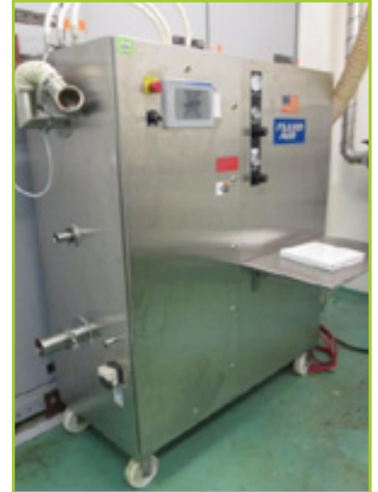
FLUID AIR MODEL 0002 XP FLUID BED DRYER WITH EXPLOSION PROOF ENCLOSURE DESIGN
