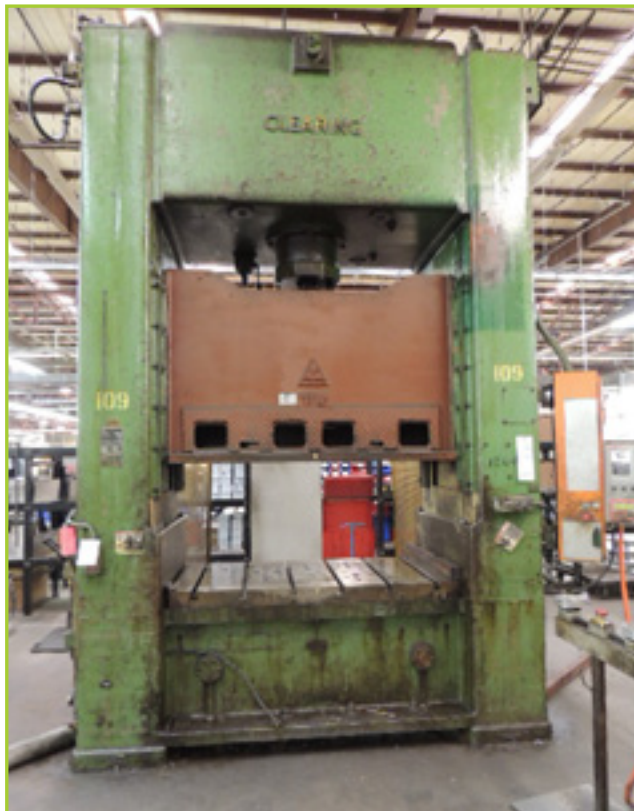
CLEARING SINGLE 175 TON PRESS, SHUT HT. ABOVE BED 22"
