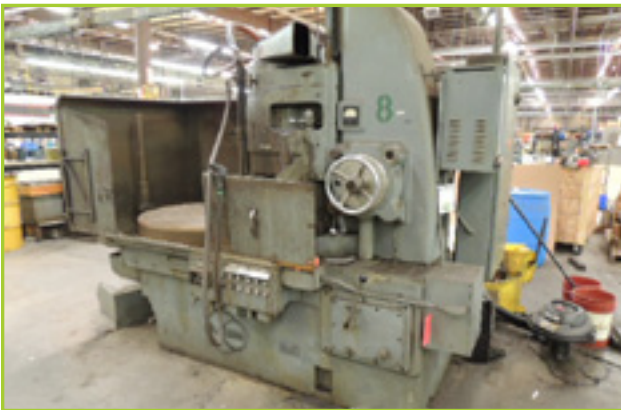
BLANCHARD NO. 18 GRINDER, 42" DIAMETER
