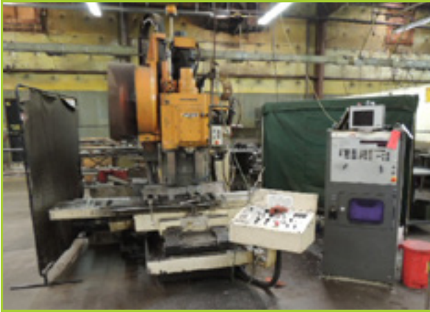
MANKINO MILL MODEL FNC-85-A20R, BED 38"X18"
