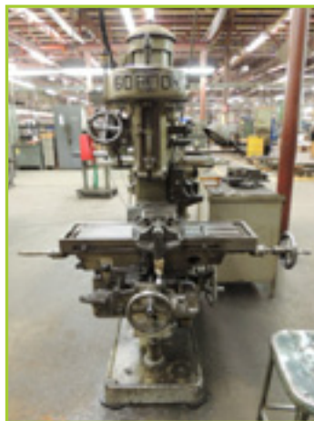
GORTON 8 1/2" D VERTICAL MILL, BED 34"X8"
