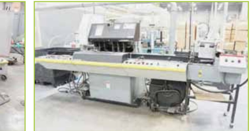
DEXTER-LAWSON PRODUCTS LTD. CLASSIC H/DCHR PAPER DRILLING MACHINE 5 HP, W/ MATERIAL HANDLER. MODEL 18CV S/N 18CV/6097. CONFIGURED FOR 2 BOOKS WITH 3 DRILLS EACH AT A TIME.
