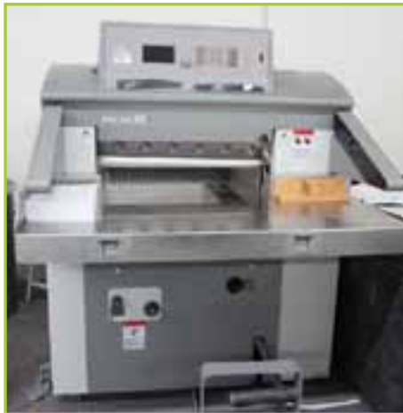
POLAR MOHR 66 PAPER CUTTER, 26.38" CUTTING WIDTH, YEAR OF MFG. 2008
