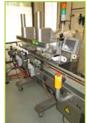
CVC TECHNOLOGIES CVC1117-2 COTTON INSERTER, MFG. 2008
