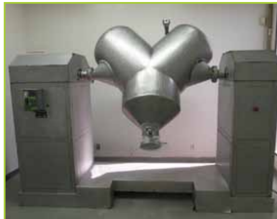
V-MIXER V-MIXER, 28 CUBIC FT. VOLUME AND NO INTENSIFIER BAR
