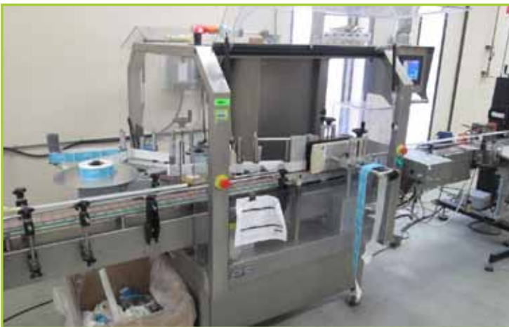
LABELER CVC TECHNOLOGIES CVC 302C LABELER, 220V, 60 HZ, 1 PH, 880W, MFG. 2007
