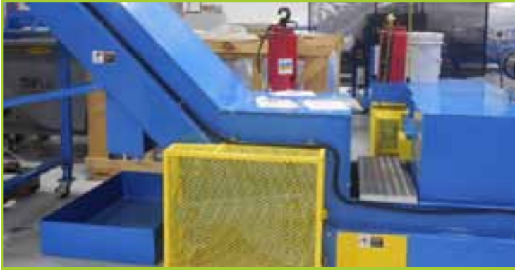
ENDURAVEYOR REJECT GLASS CULLET CRUSHER & CONVEYOR SYSTEM. [ QTY-2 IN FEED 29"W HINGED STEEL-BELT CONVEYOR TRACKS ; TRACKS APPROX. 17'L ] (GLASS CULLET CRUSHER APPARATUS 24" BELT WIDTH ; 1-HP MOTOR GEAR DRIVE AT 20'/MIN ; FOOTPRINT CRUSHER 6'LX2.5'WX2'H) (2.5 PITCH HINGED STEEL-BELT GLASS CULLET ELEVATOR CONVEYOR WITH END DISCHARGE CHUTE ; CONVEYOR 11'L ).
