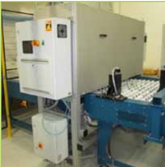
DR. SCHENK SOLAR INSPECT FLAT GLASS EDGE/SHEET INSPECT & MEASUREMENT SYSTEM , YEAR 2012. OVERALL FOOTPRINT 18'LX8'WX8'H --- SHEET WIDTH MAX 1300MM ; IN FEED ALIGNMENT CONVEYOR SECTION WITH TWO PDP LINE HEADS ; OPTICAL INSPECTION STATION WITH LED ILLUMINATORS AND TWO SC3 SMART CAMERAS (CHESS. EDGE GLASS SHEET AND EDGE DEFECT DETECTION & CLASSIFICATION ; SHEET INSPECTION SYSTEM FOR IN/ON GLASS DETECTION & CLASSIFICATION AND SQUARE-NESS ; INSPECTION UP TO 10-MICRONS) ; WITH HYFRA #CHILLY-08-C CHILLER SUPPORT ; WITH EXITING CONVEYOR SECTION. CONTROL CABINETS: (1) CONTROL CABINET WITH DR. SCHENK MAIN CONTROL COMPUTER. ALSO EV4000 WORKSTATION COMPUTER, FOR EDGE INSPECTION, IDENTIFIER AND CAMERA PROCESS. (1) CONTROL CABINET WITH DR. SCHENK EV4000 WORKSTATION COMPUTER, FOR SHEET INSPECTION. (1) CONTROLLER BOX WITH MITSUBISHI GOT-1000 OPERATOR TERMINAL, FOR ALIGNMENT/CENTERING CONVEYOR PROCESS. BLDG-ZV,FLR2,NORTH,PIF LINE.
