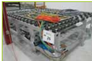
BENTELER WM4516C.01-2T0-11111-333 HORIZONTAL FLAT GLASS WASHING & DRYING SYSTEM [ YEAR 2011 ; ORDER#30-254 ; OVERALL SYSTEM FLOOR AREA FOOTPRINT 36'LX25W ; CLOSED-LOOP-SYSTEM ; SPEED 5 - 15 M/MIN FOR 0.7MM AND OVER 500X500MM PRODUCT ; 60°C HOT WATER AND DETERGENT CLEANING CAPABILITY TO REMOVE STAIN AND RESIDUE ; DI WATER INTERNAL RECYCLING CAPABILITY ; CLEAN TRANSITION INTO INSPECTION STATION], WITH EQUIPMENT: (IN FEED CONVEYOR) (QTY-48 DISK BRUSHES FOR DETERGENT WASH, WITH QTY-4 SIEMENS MOTORS ) (ROLLER BRUSHES AND SHOWER FOR DI WATER RINSE) (QTY-10 AIR KNIFE UNITS FOR DRYING) (BLOWER UNIT ON RAISED PLATFORM, OVERALL HEIGHT 15") (EXIT CONVEYOR) (INTERNAL TANKS: QTY-9 WASHING TANKS) (EXTERNAL SUPPORT: WATER POLISHING TANK SYSTEM ; FLOW VALVE ASSEMBLY RACK WITH G-MAR HEAT EXCHANGER ; H2O2 CLEANER SUPPLY TANK WITH METERING PUMP ; DETERGENT TANK WITH METERING PUMP) (REMOTE STATION: 3-SKID DI WATER FILTRATION & RECYCLING STATION WITH QTY-2 SS TANKS & QTY-2-TOTAL GRUNDFOS. TOTAL FOOTPRINT 15'LX3'W). WITH PLC CONTROL CABINET: (FOOTPRINT 14'LX7'H ; SIEMENS SEMATIC S7-300 PLC SYSTEM;SIEMENS SINAMICS A5E/6SL-SERIES DRIVES ;SIEMENS SIRIUS INDUSTRIAL CONTROLLERS ; ASSORTED RELAYS. ALSO INCLUDES QTY-1 SIEMENS TOUCH MULTI PANEL STATION)
