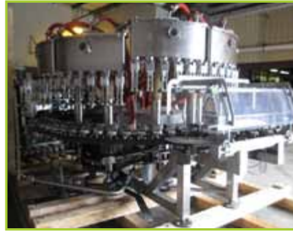
HARTNESS INTERNATIONAL FILLER BLOCK 480V, 3 PH, 60 HZ, 7.2 A FULL LOAD, S/N W2200192H
