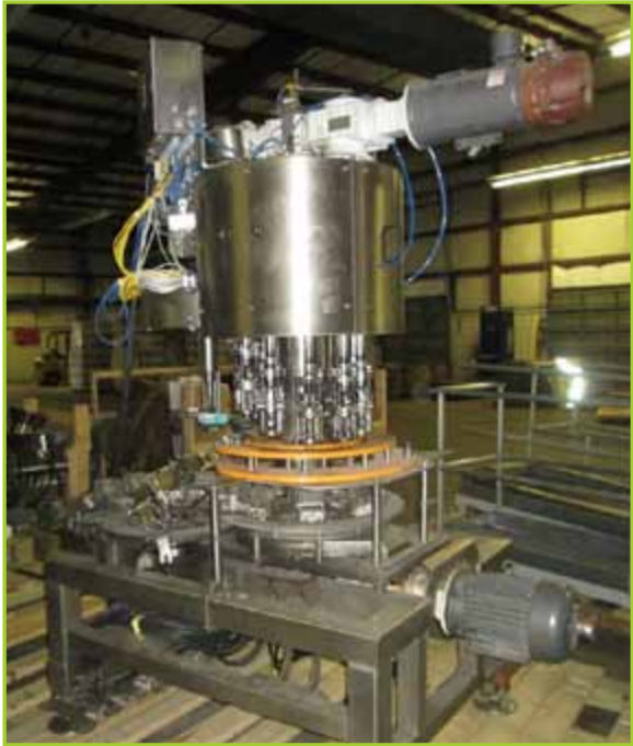
HARTNESS INTERNATIONAL FILLER BLOCK 480V, 3 PH, 60 HZ, 7.2 A FULL LOAD, S/N W2200192H
