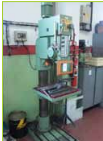
IBA EA 35 700 MM SWING VERTICAL DRILLING MACHINE WITH 9-SPINDLE SPEEDS
