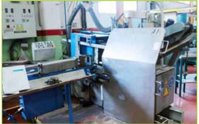
FRECH DAW 20 A SBC 20-TON HOT CHAMBER DIE CASTING MACHINE, WITH 240KN CLAMPING FORCE, 40KN INJECTION FORCE, 250MM X 250MM BETWEEN TIE BARS, 380MM X 380MM PLATEN, 180MM OPENING DISTANCE, SBC 3 CONTROLS, DISCHARGE CHUTE, RODANT MODEL OR-05 MOTORISED INCLINED STEEL BELT & SLAT FEEDER CONVEYOR 300MM WIDE ON BELT, FUME EXTRACTION FAN, FITTED WITH 12 SECTION CABLE DIE DIE AND 12 SECTION SIDE CABLE INSERTING ATTACHMENT
