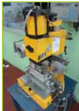
IMPAK 15 BENCH TYPE HOT STAMPING MACHINE
