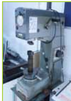
CENTAUR RB2 BENCH TYPE HARDNESS TESTER
