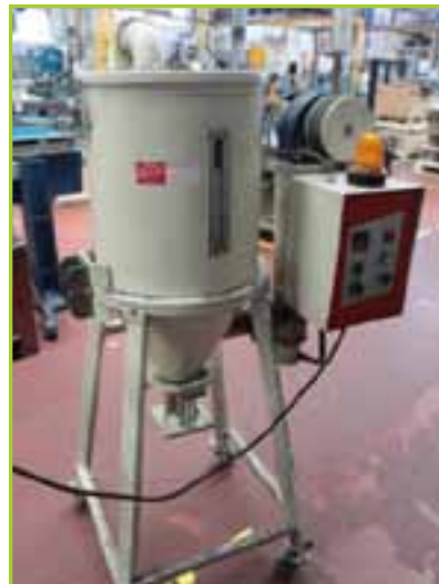
CAUFARTH D 500 MOBILE MATERIALS DRYING HOPPER
