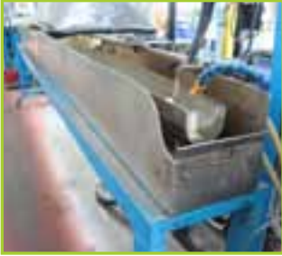
STAINLESS STEEL MOBILE COOLING BATH WITH MOTORISED PUMP
