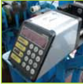
SIKORA PHOTOELECTRONIC DIGITAL DIAMETER MEASURING DEVICE
