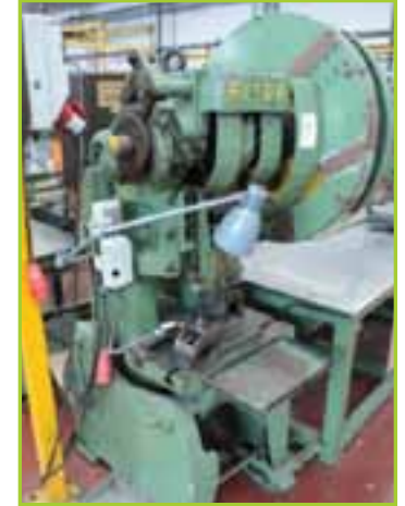
AITOR JMM 25 TON CAPACITY OPEN ENDED INCLINABLE POWER PRESS
