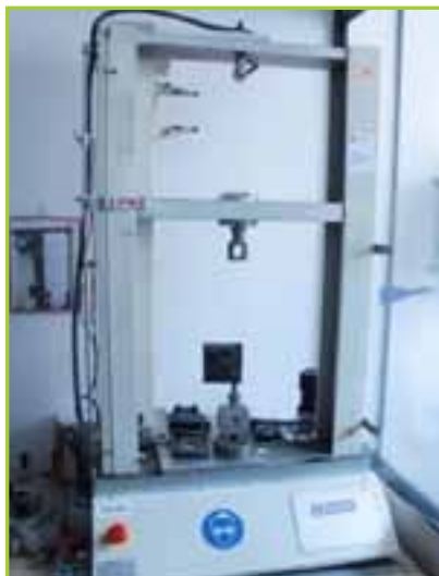
ERICHSEN 476 TENSILE TESTING MACHINE WIT TYPE DA- 630 ATTACHMENT
