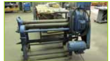
LOWN 3400 ROLLER MACHINE, 38" ROLLS
