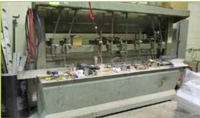
CEMCO 6-HEAD DRILLING MACHINE
