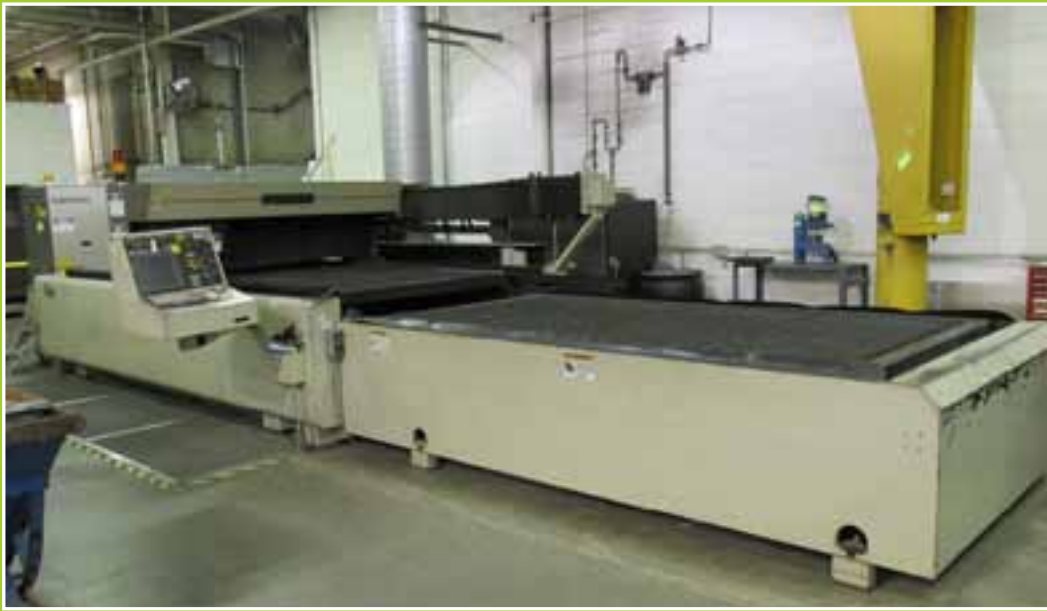
CINCINNATI CL-6 CNC LASER CUTTING MACHINE, W/ GE FANUC LASER MOD C200C, INVISIBLE: MAX OUTPUT - 5000W, PULSE DURATION 100US-CW, EMITTED WAVELENGTH 10.6UM, LASER MEDIUM CLASS IV LASER, CO2/N2/HE=5/55/40%, VISIBLE: L5MW, CW, 0,6-0.7UM, W/ 2-TRANSFORMERS, KOOLANT KOOLERS
