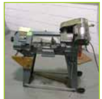
RF MBS-92285B METAL CUTTING BAND SAW
