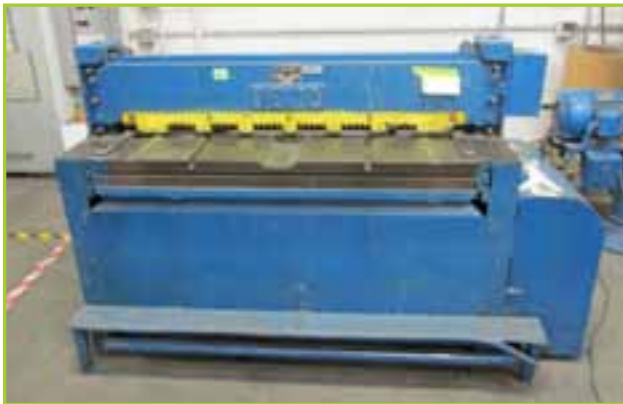
PEXTO 12-U-4J SHEAR, 49"W CAP, 12-GA SOFT STEEL CAP
