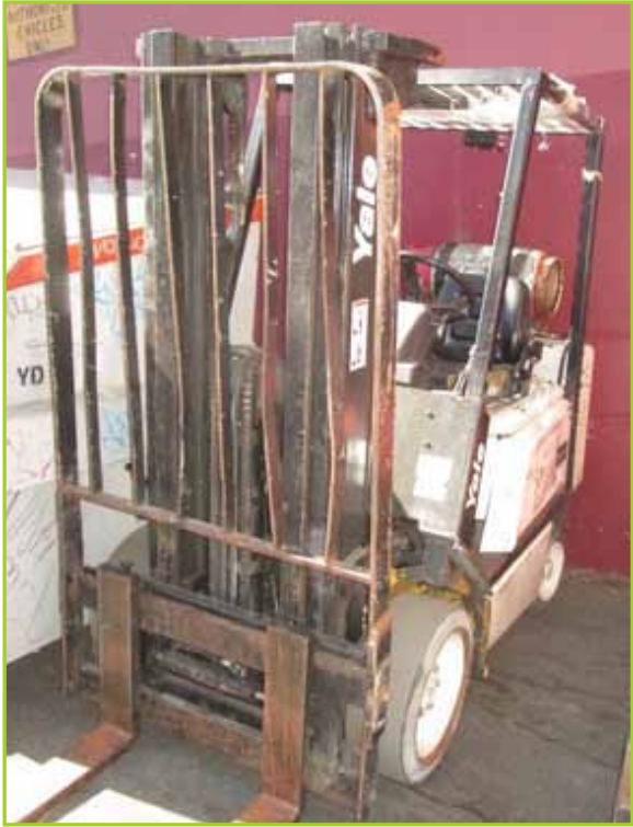
YALE GLC050TENUAE083 FORKLIFT PROPANE STYLE, CAPACITY 5000 LBS., METER 12706 HRS., 36" FORKS
