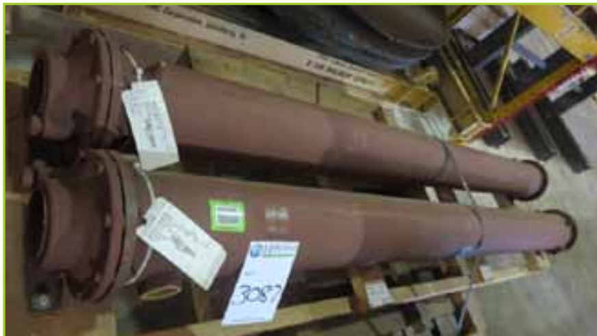
HEAT EXCHANGER API HEAT TRANSFER 1503-06-078-001 LOT CONTAINS 2 HEAT EXCHANGERS, BASCO, SPECIAL TYPE 500, 1 PASS ASSEMBLY, 3/8" TUBES, 3" SPA, DATE OF MFG. 6/2011
