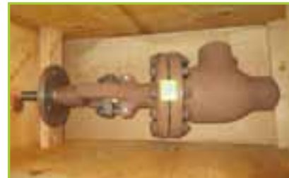
VALVE CRANE-ALOYCO INC CA00705 VALVE, AC 3"600 180-1/2U.A216 WCB BODY, BWE
