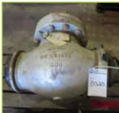
CRANE-ALOYCO INC 175-1/2X VALVE , DC 8"600 175-1/2X CS.
