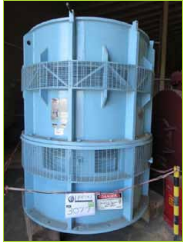
SQUIRREL CAGE INDUCTION MOTOR ELECTRIC MACHINERY HEAVY DUTY MOTOR, PUMP, 2000 HP, 3 PH, 4000V, 60 HZ, 1185 RPM, 5523V FRAME, CL. B NS, 1.15 SF, 250 AMP
