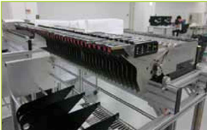
FUJI NXT KT08B 8MM FEEDERS, BUCKET TYPE
