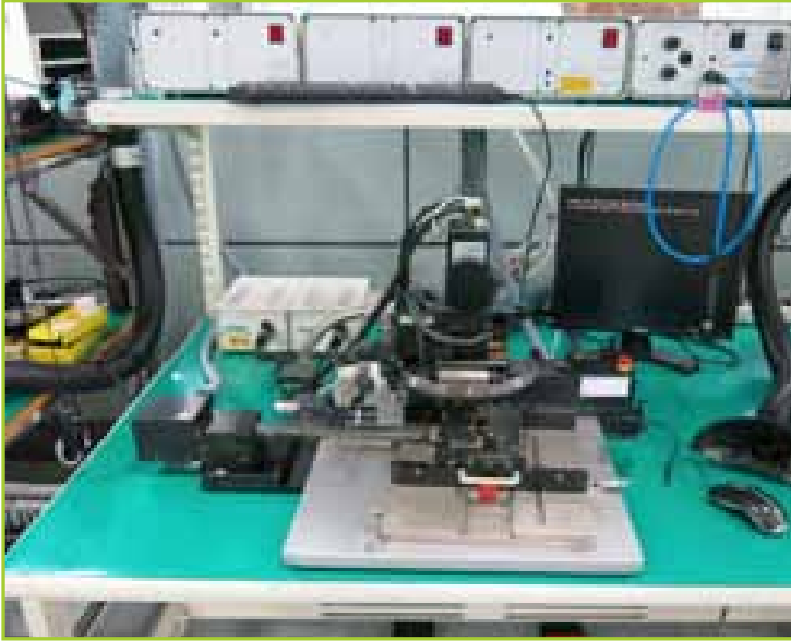
FINETECH PICO FINETECH PICO HIGH DENSITY REWORK STATION
