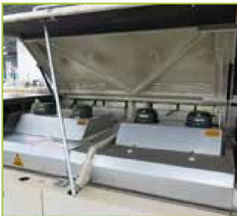
ERSA HOTFLOW 2/14 FLOW DIRECTION: LEFT TO RIGHT; HEATING ZONES: TOP 7/BOTTOM 7; COOLING ZONES: TOP 2/BOTTOM 2; NITROGEN EQUIPPED; EDGE RAIL BOARD TRANSPORT ; CENTER BOARD SUPPORT; AUTO OILER; WATER COOLING; DUAL LANE. S/N: R009A-05C0172. MANUFACTURED IN 2005
