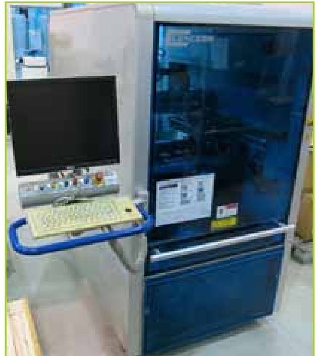
CENCORP 1000 BR IN-LINE BOTTOM ROUTER WITH EXTERNAL VACUUM SYSTEM
