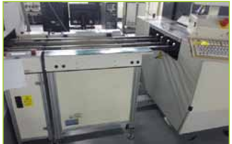
EUNIL EWT-100 INSPECTION CONVEYOR, LENGTH (MM) 1100; MIN WIDTH 30 (MM); MAX WIDTH 205 (MM) ; DUAL LANE
