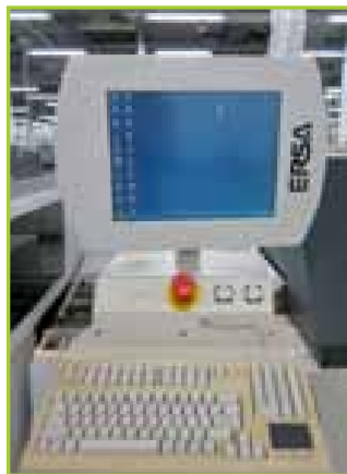
ERSA HOTFLOW 2/14 FLOW DIRECTION: LEFT TO RIGHT; HEATING ZONES: TOP 7/BOTTOM 7; COOLING ZONES: TOP 2/BOTTOM 2; NITROGEN EQUIPPED; EDGE RAIL BOARD TRANSPORT ; CENTER BOARD SUPPORT; AUTO OILER; WATER COOLING; DUAL LANE. S/N: R009A-05C0172. MANUFACTURED IN 2005
