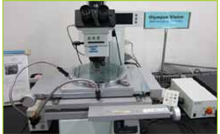
OLYMPUS STM6-LM-F31-2 COMPACT MANUAL 3-AXIS MEASURING MICROSCOPE, 2006
