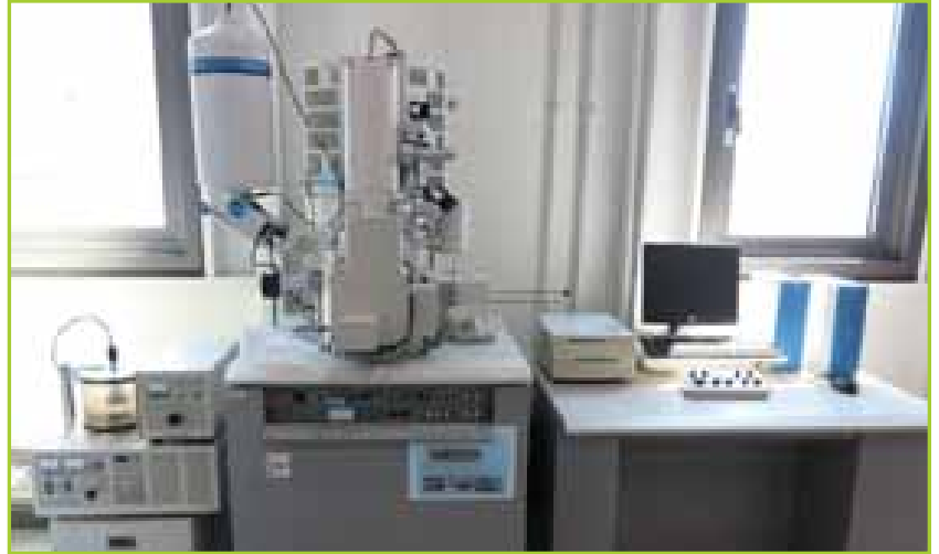
HITACHI S-4700 THE HITACHI S-4700 IS A FIELD EMISSION SCANNING ELECTRON MICROSCOPE (FE-SEM), UNDER OPTIMAL CONDITIONS, CAN MAGNIFY IMAGES UPWARDS OF 500,000 TIMES AND RESOLVE FEATURES TO 2 NANOMETERS. IN ADDITION, A CATHODOLUMINESCENCE DETECTOR, MANUFACTURED IN 2006.
