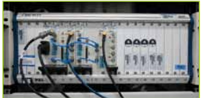
AEROFLEX 82547 18 SLOT PXI CHASSIS WITH MXI INTERFACE
