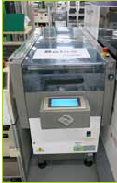
JOT DISTRIBUTION CONVEYOR, (MM) 500; MIN WIDTH 50 (MM); MAX WIDTH 200 (MM) ; TRIPLE LANE
