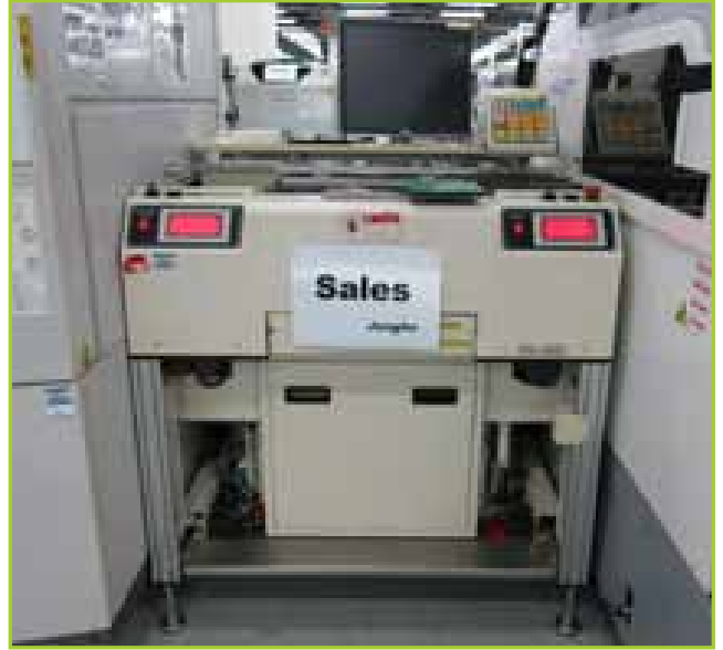
EUNIL EGC-300D SHUTTLE GATE CONVEYOR, LENGTH (MM) 1300; MIN WIDTH 30 (MM); MAX WIDTH 205 (MM) ; DUAL LANE
