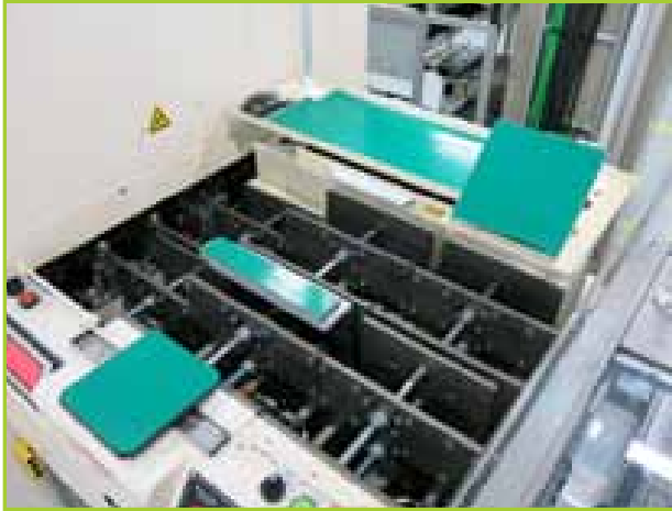
EUNIL ENC-800D INSPECTION CONVEYOR, LENGTH (MM) 1000; MIN WIDTH 30 (MM); MAX WIDTH 205 (MM) ; DUAL LANE
