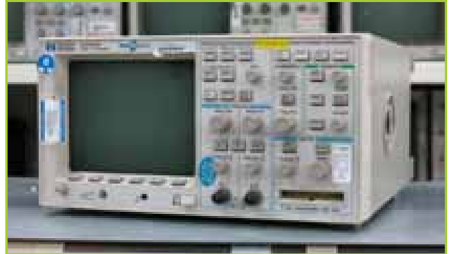
HEWLETT PACKARD 54645D 100-MHZ SCOPE WITH 200 MSa/s, 1 MB OF MEMORY PER SCOPE CHANNEL, 16 LOGIC TIMING CHANNELS WITH 400 MSa/s ON 8 CHANNELS, 200 MSa/s ON 16 CHANNELS, 2 MB OF MEMORY PER LOGIC CHANNEL, AGILENT MEGAZOOM TECHNOLOGY ALLOWS DEEP MEMORY CAPTURE
