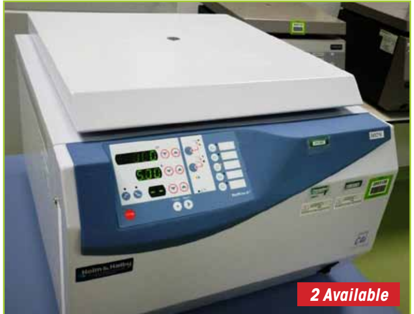
JOUAN C41 MOBILE CENTRIFUGE , CHAMBER DIA 450MM, MAX SPEED 7800 RPM, MAX LOAD 3.6KG AT 4000RPM, 230 VOLTS WITH DIGITAL CONTROLS AND MOUNTED ON MOBILE TABLE. YEAR 2007
