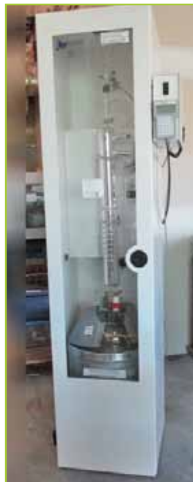
B/R INSTRUMENTS 9600 HPLC ACETONITRILE DISTILLATION SYSTEM, IN CABINET ENCLOSURE; YEAR-2009
