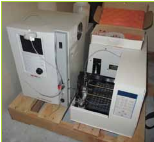
MATEC APPLIED SCIENCES CHDF-2000 CAPILLARY HYDRODYNAMIC FRACTIONATION, PARTICLE SIZE ANALYZER (SIZE DIAMETER MEASUREMENT 15-NANOMETERS TO 1.1 MICRONS). WITH MODEL-719/00000/11M AUTOSAMPLER-INJECTOR. WITH MODEL-C-202-L FRACTIONATION CARTRIDGE
