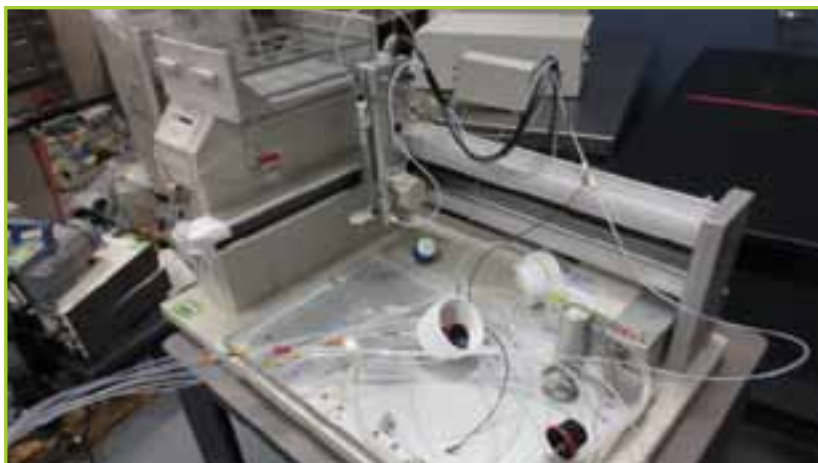
WATERS 1- DELTA 600 PUMP, 1- GILSON 215 LIQUID HANDLING SYSTEM, 1- WATERS UV FRACTION MANAGER, 1- 600 CONTROLLER, 1- 2487 DUAL ABSORBANCE DETECTOR
