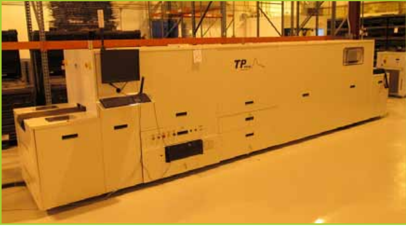
TP SOLAR D-225L INFRARED FURNACE , 480V 3 WIRE/NEUTRAL/GROUND, 50/60 HZ, 85 KW, 101 AMPS, 75 PSI, 19 LPM@ 4 BAR, 1500 SCFH, PROCESS EXHAUST 350 SCFH, CABINET EXHAUST 500 SCFH, 10" X 238" WIRE CONVEYOR. SN# 2011189. YEAR: 2010
