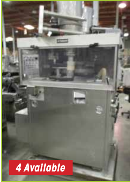
STOKES 328-1 ROTARY TABLET PRESS , 35 STATION, 10 TON COMPRESSION
