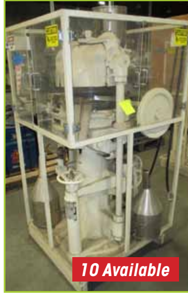
STOKES BB2 ROTARY TABLET PRESS , 30 STATION, 4.4 TON RELEASE PRESSURE
