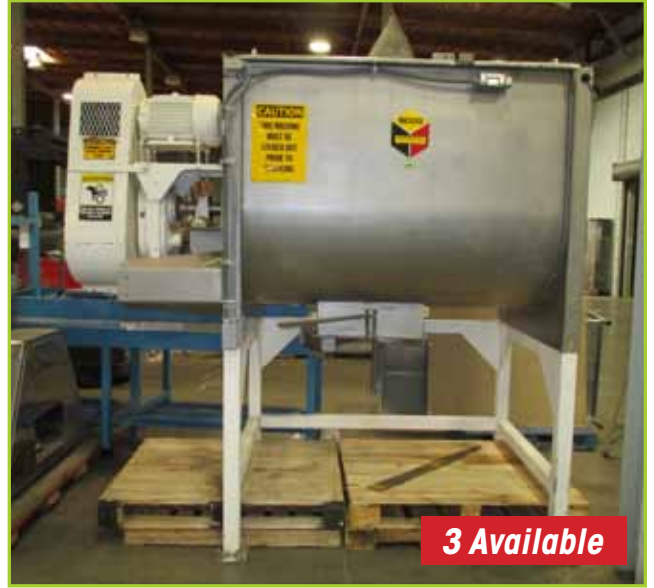
SCOTT EQUIPMENT CO. SHRM384 RIBBON BLENDER WITH HARD WIRED ELECTRIC MOTOR AND SHAFT MOUNTED SPEED REDUCER
