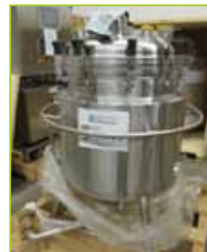
T&C STAINLESS 250 L JACKETED STAINLESS STEEL VESSEL
