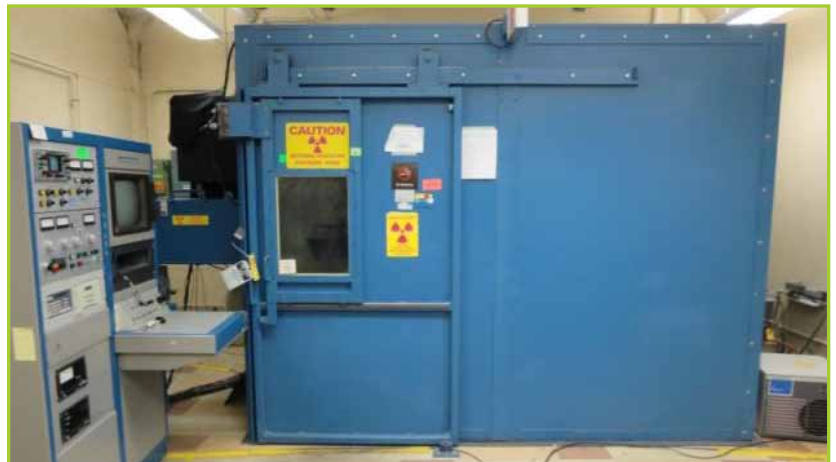
TFI MCP160H X-RAY SYSTEM MICROFOCUS REAL TIME. WITH CTI-CRYOGENICS 8200 COMPRESSOR & BERNARD VACUUM PUMP
