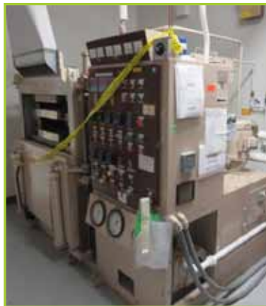
WALBASH METAL PCV80-18183CTMX LAMINATOR PRESS 18"X18"
