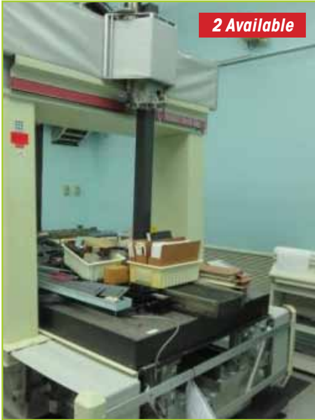
SHEFFIELD CORDAX RS-70 COORDINATE MEASURING MACHINE W/CONTROLLER. WITH RENISHAW PROBE HEAD CONTROLLER, AUTO CHANGE CONTROL UNIT & AUTO CHANGE CONTROL UNIT
