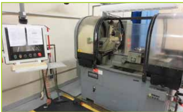
HARDINGE 16 CHCN BAR & CHUCKING MACHINE. COMPUTERIZED NUMERICAL CONTROL BAR AND CHUCKING MACHINE
