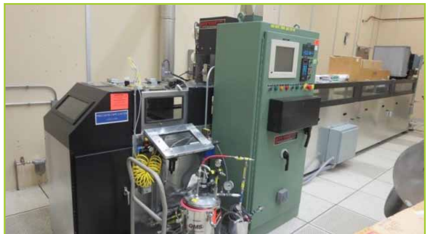
PROCAST CONTINUOUS TAPE CASTING MACHINE. PRECISION TAPE CASTER WITH SPARE PARTS & MANUAL
