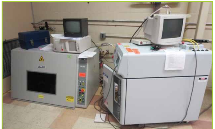
UNITEK MYACHI LW100 YAG LASER WELDING SYSTEM. WITH SCHREIBER CHILLER MODEL 150AC
