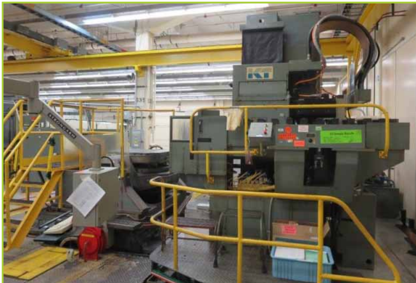
KEARNEY & TRECKER TRAVELING COLUMN MODU-LINE MACHINING CENTER 5 AXIS WITH KT/CNC CONTROL
