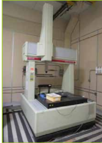
GIDDINGS & LEWIS RS-70 MACHINE CORDAX MEASURING MACHINE
