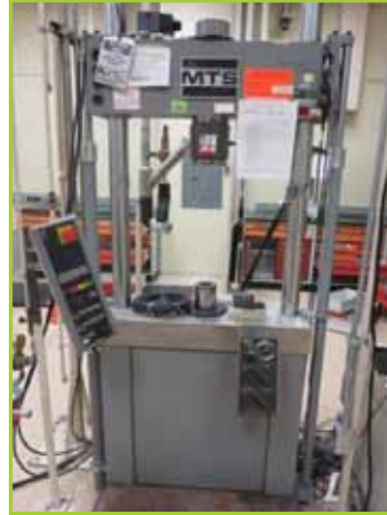
MTS LOAD FRAME 25TON /55 WITH OSCIL- LOSCOPE & MTS TEST STAR II
