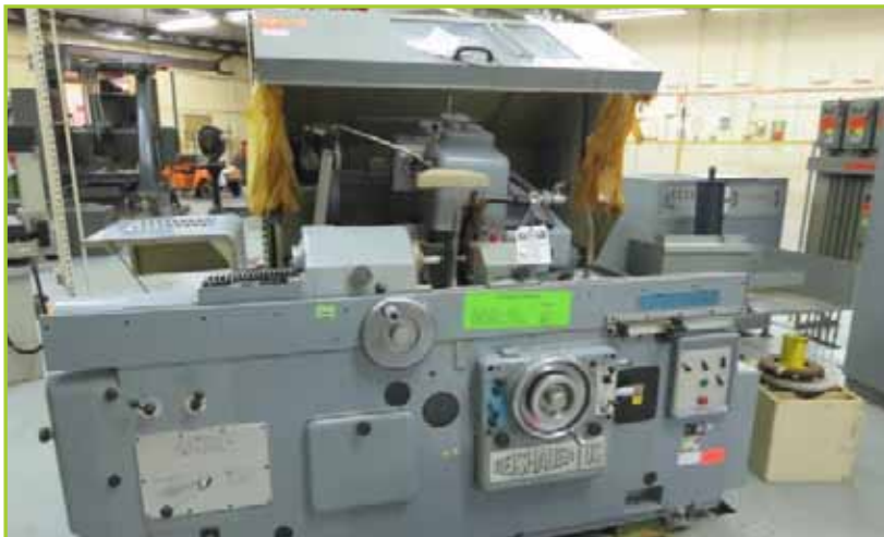
REISCHAUER TYPE US THREAD GRINDER. WITH OIL COOLER, EXTRA GRINDING WHEELS, BOX & CART OF CHANGEABLE GEARS
