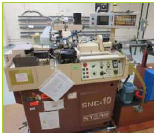
STAR SNC-10 AUTOMATIC SCREW MACHINE WITH STAR YASNAC 2000G POWER SUPPLY
