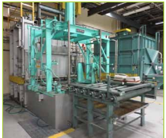
SECO/WARWICK CORP N/A HEAT TREAT FURNACE. MAX CAPACITY 925LB , OPERATING TEMPERATURE 1000° F , WITH EXIT ROLLERS AND TANK
