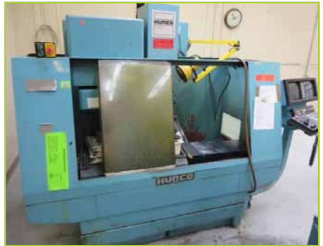
HURCO BMC20 CNC VERTICAL MILLING MACHINE
