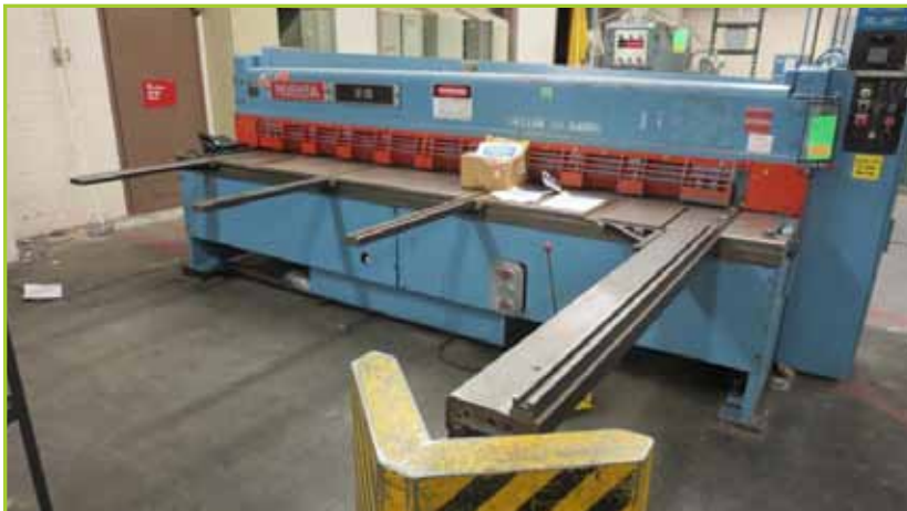
NIAGARA IF-10 10' SHEAR. HYDRAULIC SHEAR, UNDER DRIVE SERIES 1/8 MILD STEEL
