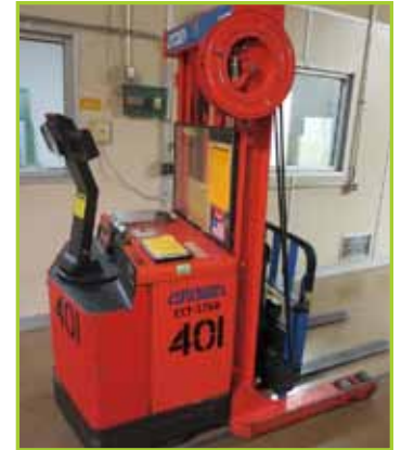
CROWN 30WR7LS WALKIE STACKER FORK TRUCK. CAPACITY 3000 LBS. MAX HEIGHT 116"
