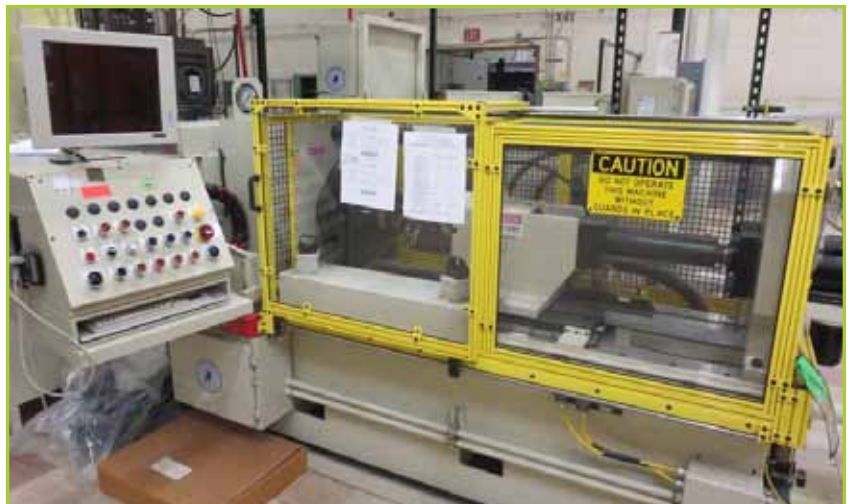
MT MANUFACTURING 180B FRICTION INERTIA WELDER
