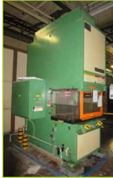
CINCINNATI MILACRON 175 HYDRAULIC PRESS. 175 TON MAX STROKE 10"
