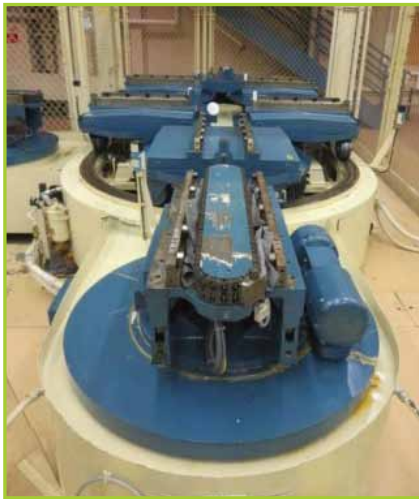
KEARNEY & TRECKER N/A PALLET POOL 6 POSITION. WITH TRIAD LIGHT CURTAINS
