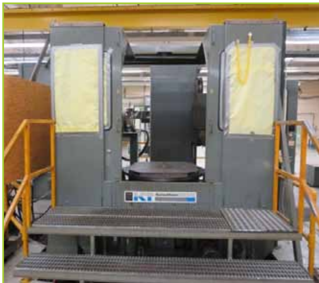
KEARNEY & TRACKER MODU-LINE CNC MACHINING CENTER 5-AXIS
