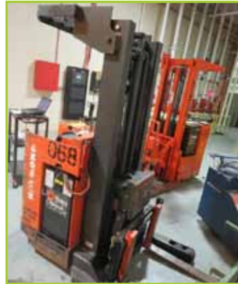
RAYMOND ENGINEERING 20R30TT ELECTRIC LIFT TRUCK. CAPACITY 3000LBS
