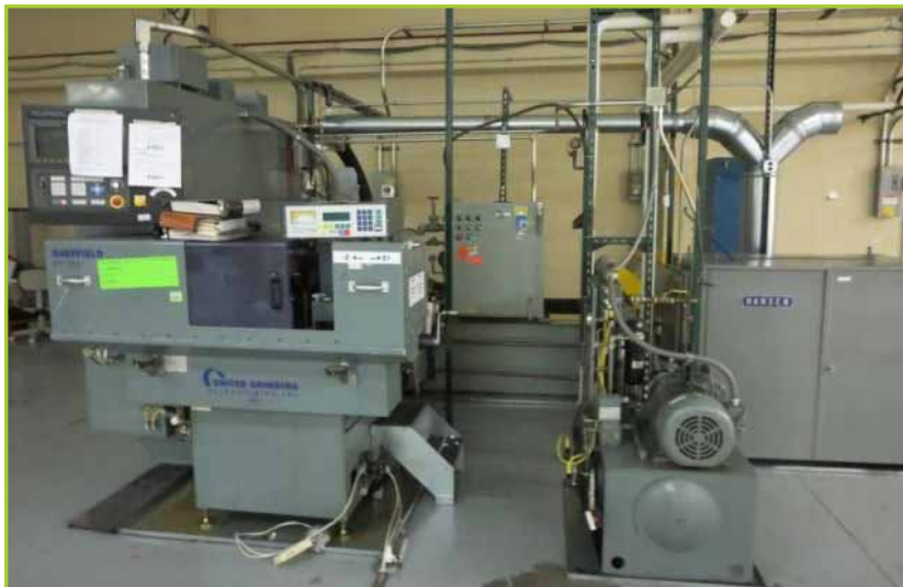
SHEFFIELD 5WT1P1C O-GC CRUSHER GRINDER WITH SMOG HOG INDUSTRIAL AIR CLEANER, HANSON CHILLER MODEL # 5WT1P1C, AIR FLOW MIST COLLECTOR
