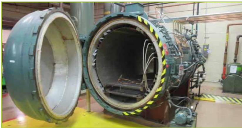
BARON & BLAKESLEE BVAC-58 AUTO CLAVE. WITH BEACH RUSS SIZE 150-D VACUUM PUMP
