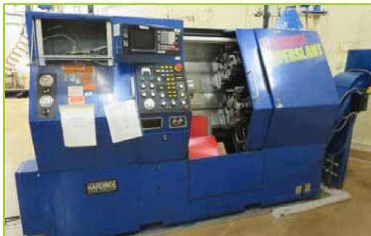
HARDINGE SB-4GN SUPERSLANT CNC LATHE. WITH RETRACTABLE BAR FEED
