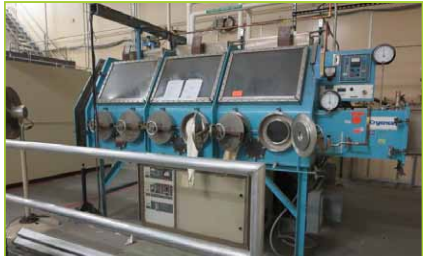
MERRICK 106487/3 VACUUM CHAMBER GTA WELDER WITH VAC DRY INERT ATMOSPHERE MODEL M040-2, LEYBOLD ROTARY VANE PUMP, (ROCKY #000-21956-91914-00), PLAT FORM STAND AND WELD CURTAIN
