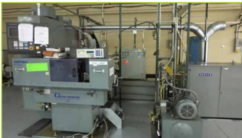
SHEFFIELD 5WT1P1C O-GC CRUSHER GRINDER WITH SMOG HOG INDUSTRIAL AIR CLEANER, HANSON CHILLER MODEL # 5WT1P1C, AIR FLOW MIST COLLECTOR
