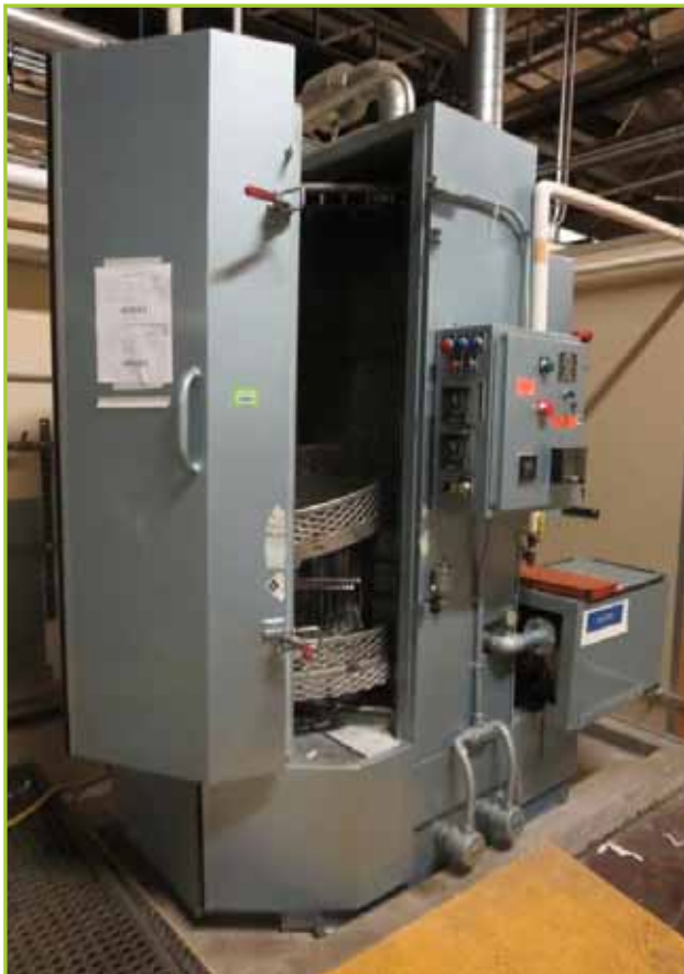
BETTER ENGINEERING 300LX AQUEOUS SPRAY CLEANER. PARTS CLEANER PRESSURE JET STEAM CLEANER. S/N- 8307. YR. 1992
