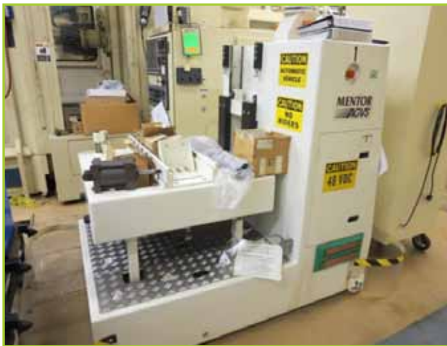
MENTOR M036672 VEHICLE AUTO GUIDED SYSTEM. LOAD WEIGHT 1500LBS. 48VOLT WITH BATTERY & CHARGER
