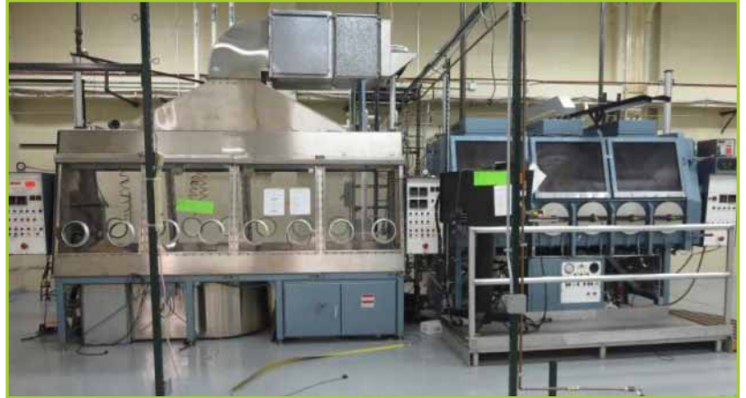
TM VACUUM PRODUCTS ARC WELDER. WITH GLOVE BOX SYSTEM
