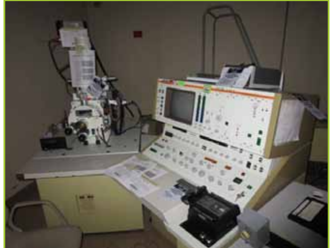
ELECTRIC SCANNING MICROSCOPE. WITH TV SYNCHRONIZATION GENERATOR & ELECTRON CATHODE GUN WITH ION PUMP
