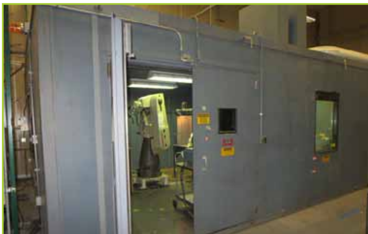
UNIMATE PUMA 762 ROBOT SPRAY BOOTH W/FLAME. UNIMATE PUMA 700 ROBOT METCO BOOTH IS16FT W X 22FT L X 9FT H
