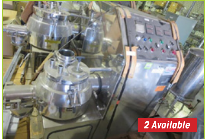
POWREX FM-VG-25 HI SHEAR VERTICAL GRANULATOR. STAINLESS STEEL CONSTRUCTION 15L NET CAPACITY, WITH VARIABLE SPEED IMPELLER FROM 60-500 RPM AND CROSS-SCREW SPEED FROM 360-3600 RPM, 120/220V. YEAR NEW: 1997
