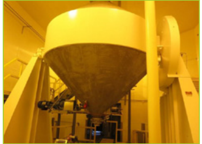
THOROBLENDER. 10' DIA. WELDED CONSTRUCTION, BUILT IN DELUMPER, MATERIAL: ALL PARTS CONTACTING PRODUCT 316 L.S.S., INTERIOR FINISH: P2 SEMI POLISH FINISH, TOTAL VOLUME 454 CU. FT., WORKING VOLUME 320 CU. FT. @80LBS CU.FT. DENSITY. TOTAL EST. WT. 18,950LBS, VESSEL DESIGNED FOR 2" HG INTERNAL VACUUM, BLENDER SPEED 12.9 R.P.M. WITH 28" W X APPROX 25FT OF CONVEYOR & STAIRS & CAT WALK SURROUNDING BLENDER.
