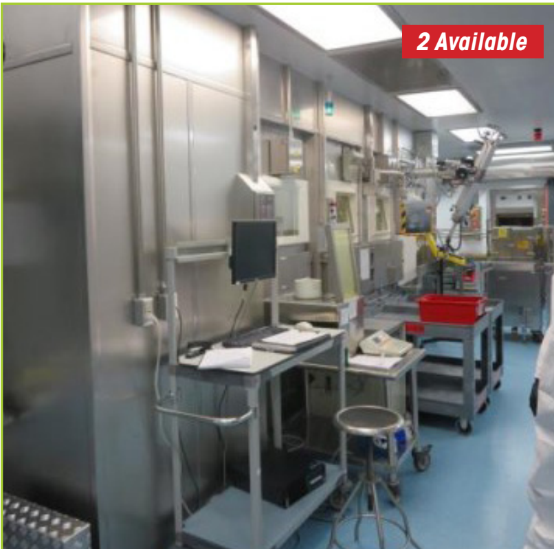
BAUSCH TYPE 534 THE BAUSCH TYPE 534 FILLING MACHINE IS PRIMARILY DESIGNED FOR DOSING CONTAINERS. THE CONTAINER TRANSPORT SYSTEM CONSISTS OF A ROTARY INFEED TABLE, A WALKING BEAM TRANSPORT, AND A ROBOT ASSISTED DISCHARGE. EXPOSED SURFACES OF THE EQUIPMENT ARE COMPOSED OF 316L STAINLESS STEEL OR OTHER CORROSION RESISTANT MATERIALS (NON-METALLIC). AN ALLEN BRADLEY CONTROL LOGIX PLC CONTROLS THE TYPE 534. ENTERING PARAMETERS AND MACHINE SPEEDS, VIEWING FAULT MESSAGES, AND OPERATING OF THE MACHINE ARE PERFORMED USING THE AB VERSAVIEW TOUCH SCREEN. THE MACHINE IS CURRENTLY CONFIGURED TO FILL 10ML SERUM VIALS WITH FILL RANGES OF 1.1 ML TO 9.9ML VIA A FLEXICON PD121 PUMP. CHANGE PARTS ARE AVAILABLE FROM BAUSCH FOR OTHER VIAL SIZES. THE SEQUENCE OF THE INDIVIDUAL STEPS IS AS FOLLOWS: CONTAINER REGISTRATION; GAS FLUSHING WITH VACUUM EXTRACTION; CHECKING FOR SUFFICIENT GAS AND VACUUM LEVELS; CONTAINER DOSING; CONTAINER CLOSING WITH STOPPER AND CHECKING FOR THE PRESENCE OF A STOPPER; CAP PLACEMENT AND CHECKING FOR THE PRESENCE OF A CAP; CONTAINER CLOSING WITH CRIMP CAPS AND CHECKING FOR THE PRESENCE OF A CAP; CAPINTEC TRANSFER; CONTAINER DISCHARGE/REJECT/SAMPLING
