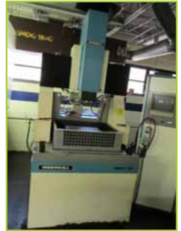
INGERSOLL GANTRY 500 GANTRY TYPE EDM MACHINE, 3R TOOLING, REMCOR CHILLER
