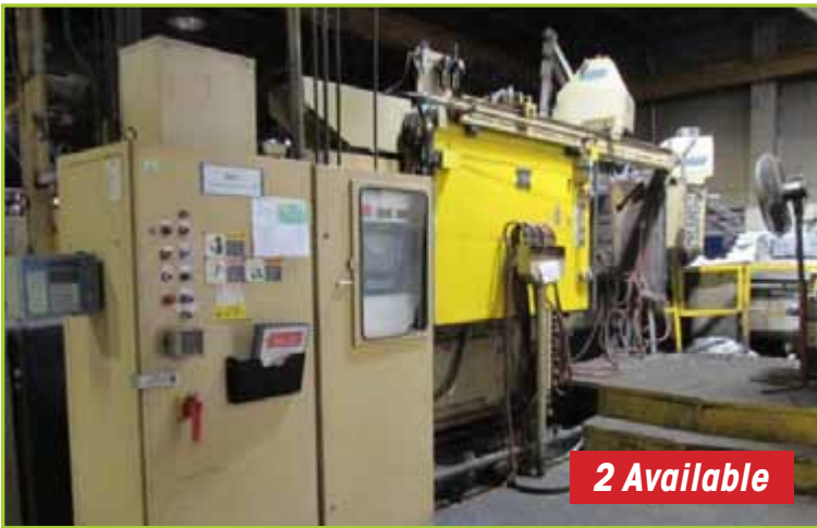
IDRA 01560 COLD CHAMBER DIE CAST MACHINE , 600-TON, ALLEN BRADLEY PLC5 CONTROLS, W/ PANEL VIEW SN# 7005. YEAR: 1996
