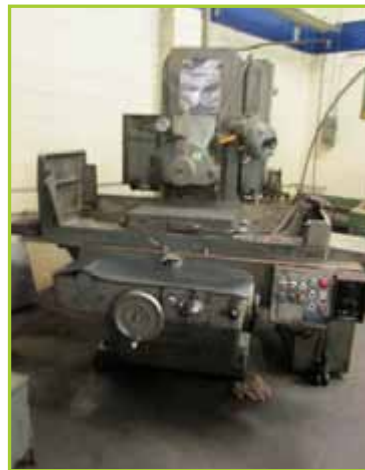
GALLMEYER & LIVINGSTON 470 HYDRAULIC SURFACE GRINDER, 12" X 24" MAGNETIC CHUCK
