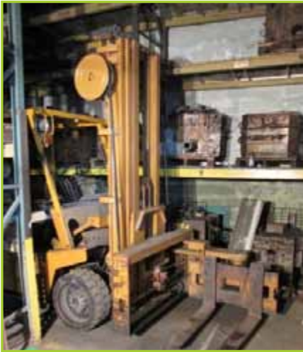
KOMATSU FG35SI TYPE G LIFTTRUCK, 14,000LB CAP, SIDE SHIFT, SOLID TIRES
