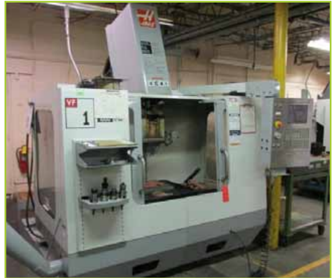
HAAS VF1D CNC DRILL/TAP MACHINING CENTER, 20-HP, VECTOR DUAL DRIVE, 1000IPM, 0 -7500 SPINDLE SPEED, 14" X 26" TABLE, 20+1 TOOL CHANGER, FEEDRATES: 0 TO 650IPM, TRAVELS: X- 20", Y-16", Z- 20", CNC CONTROLS, BT30 TAPER, AUGER CHIP CONVEYOR, YEAR: 2006
