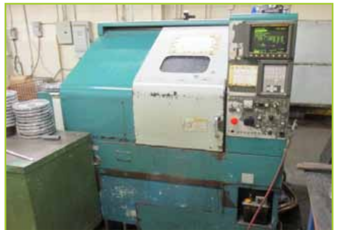
NAKAMURA TMC-18 CNC LATHE, 2-AXIS, CHUCK SIZE 8", SWING 15.74", BAR CAP 2", MACHINING LENGTH 12", 15-HP, 4500 RPM
