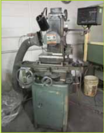
HARIG 612 SURFACE GRINDER, W/ ACU-RITE CONTROLS, 6" X 12" MAGNETIC CHUCK
