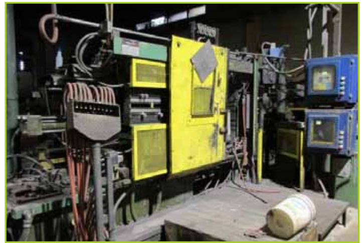
HPM II-400-A COLD CHAMBER DIE CAST MACHINE , 400-TON, RELAY LOGIC CONTROLS SN# 88010. YEAR: 1988
