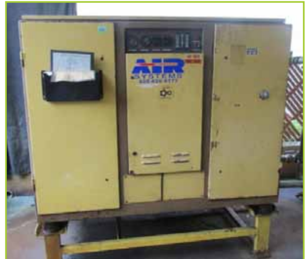
KAESER CS120 ROTARY SCREW AIR COMPRESSOR, 100-HP, 390 CFM, REBUILT 2008
