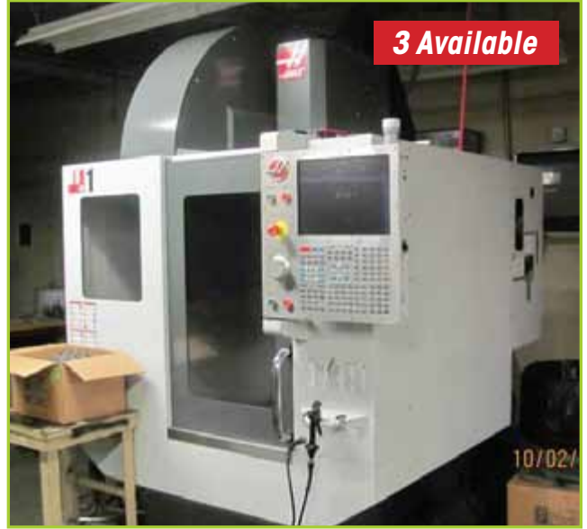
HAAS DT-1 CNC DRILL/TAP MACHINING CENTER , 15,000 SPINDLE SPEED, 15-HP, 15" X 26" TABLE, 20+1 TOOL CHANGER, FEEDRATES: MAX RAPIDS 2400 IPM, MAX CUTTING 1200 IPM, TRAVELS: X- 20", Y-16", Z- 15.5", CNC CONTROLS, BT30 TAPER, AUGER CHIP CONVEYOR, AUTO AIR GUN, RENISHAW WIRELESS TOOL-SETTING PROBE, YEAR: 2011
