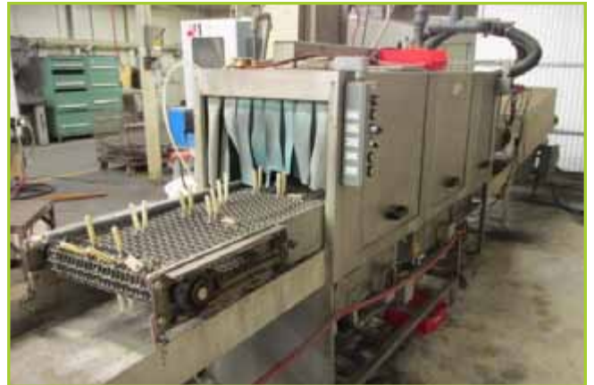
CHAMPION PARTS WASHER & DRYER , WASHER 18" X 141", DRYER 14" X 72". WASH TEMP 140 DEGREE F. FINAL RINSE 140 DEGREE F, CHLORINE 50PPM, FINAL RINSE 20PPM
