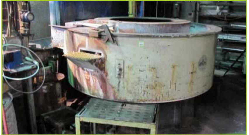
SWECO FMS20 LR VIBRATORY TUB FINISHER , 20 CU FT YEAR: 1987
