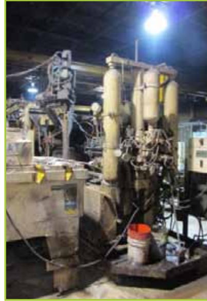
IDRA OL560 COLD CHAMBER DIE CAST MACHINE , 560-TON, ALLEN BRADLEY PLC5 W/ PANEL VIEW CONTROLS
