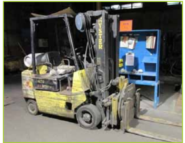
HYSTER S50XL LIFT TRUCK, 4750LB CAP, SIDE SHIT, SOLID TIRES, LPG, W/ SWIVEL FORK ATTACHMENT
