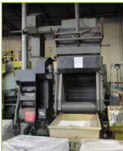
GOFF 12FD TUMBLE BARREL BLAST MACHINE, 12 CU FT
