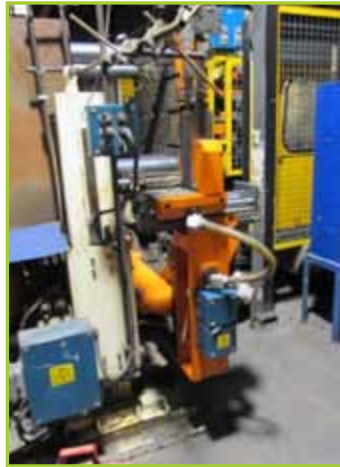
EPAC2 ROBOT, STROKE 70", 38LB CAP, W/ ALLEN BRADLEY SLC5104 CONTROLS
