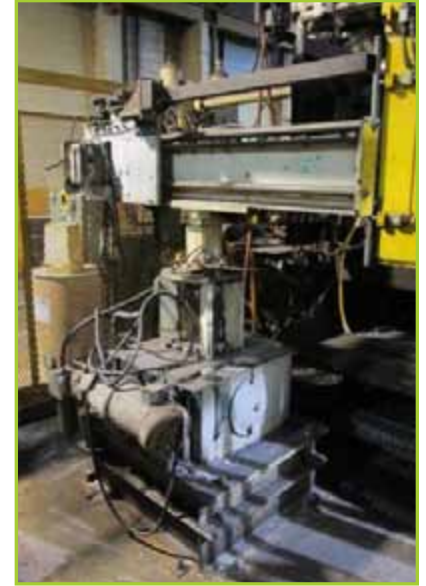
RIMROCK 195 RECIPROCATOR , W/ RELAY LOGIC CONTROLS, 55" STROKE YEAR: 1991
