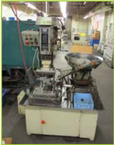
SGM DRILLING & TAPPING STATION, W/ 21" VIBRATOR BOWL FEEDER & 7" POWER CHIP CONVEYOR
