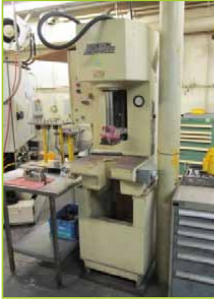
DENISON S085LC2 MULTIPRESS , 8-TON, 5-HP, 18" DAYLIGHT, 7" THROAT, 2.25" RAM DIA
