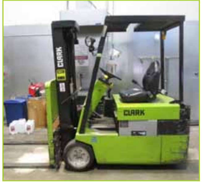
CLARK TM25 36 VOLT ELECTRIC FORKLIFT S/N TM247 0809 9055 WITH SIDESHIFT, MAST: THREE STAGE, TYPE: SITDOWN 3 WHEEL, HOURS 3734, 48" FORKS, WITH TROJAN II 36 VOLT CHARGER, MODEL 18T875C22
