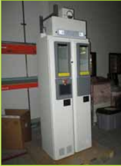
SEMIGAS DUAL TANK GAS CABINET, SILANE
