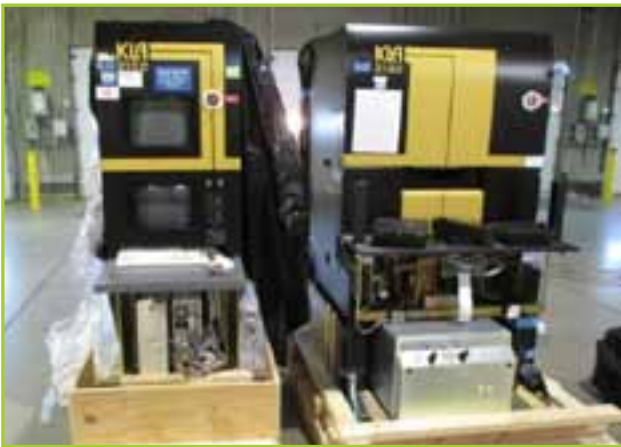
KLA-TENCOR 2132 WAFER DEFECT INSPECTION SYSTEM , THROUGHPUT ~ 2-8 WPH, 4\", 5\" & 6\" WAFER CAPABLE
