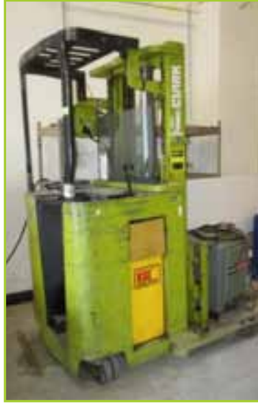
CLARK NP300-30B NARROW AISLE 24V UPRIGHT ELECTRIC FORKLIFT, MAX 1600LBS
