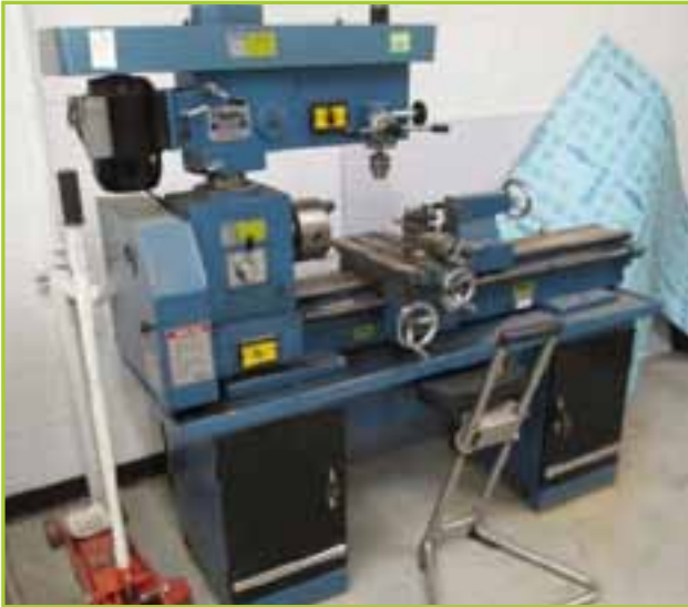
SMITHY CB-1239 LATHE/MILL MACHINE
