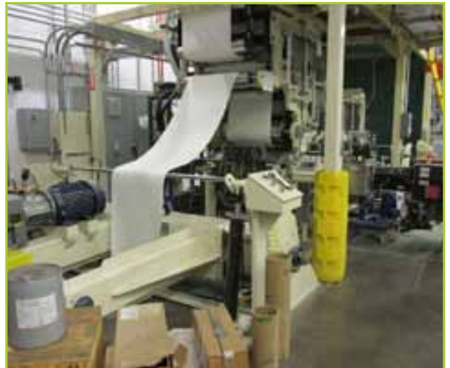
RETROFLEX SLOT DIE COATER ROLL STAND , W/ UNWIND-REWIND CAP., STEEL MAIN FRAME & ROLL FRAMES, SLOT DIE SUPPORT AND POSITION SETTINGS, BACK UP ROLL, ALIGNMENT ROLL, CHILL ROLLS, COATING STATION DRIVE SYSTEM, SMOOTHING ROLL, STATIC BAR, GUIDE ROLLS, STERLING GPAC-30 CHILLING UNIT, 3-STERLING MZB2020-C TEMP CONTROL UNITS, WEB GUIDES, DEGAUSSING BAR, 5-SET FIXED SLOT HOT MELT COATING DIES, 4-POSTION DISPLACEMENT GEAR MELT PUMPS - TYPE 36/36-01, CONTINUOUS SCREEN CHANGER - TYPE K-SWE-121 . YEAR 2011
