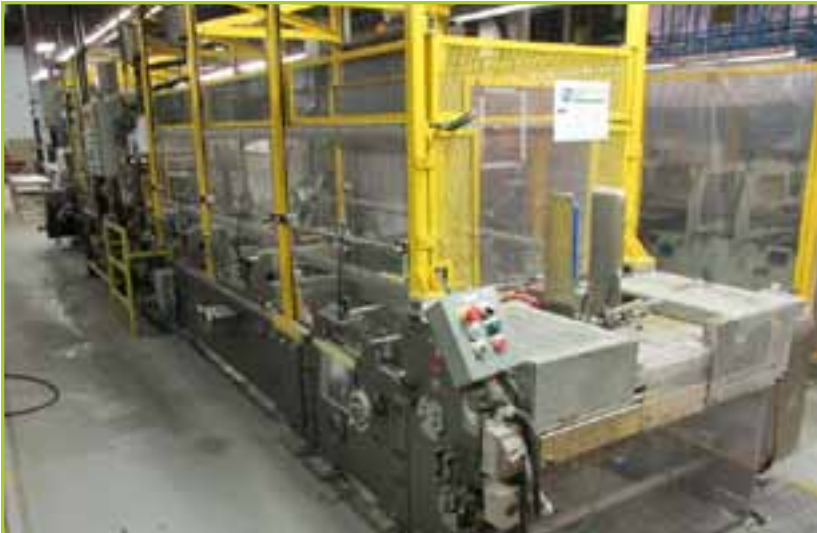
WESTERN SLOPES KF ROYAL 333 FLAME SEALER , LINE SPEED 1,500 BFPM, CARTON RANGE LENGTH 2.5" TO 33", CARTON RANGE WIDTH 7.25" TO 33". YEAR 2006
