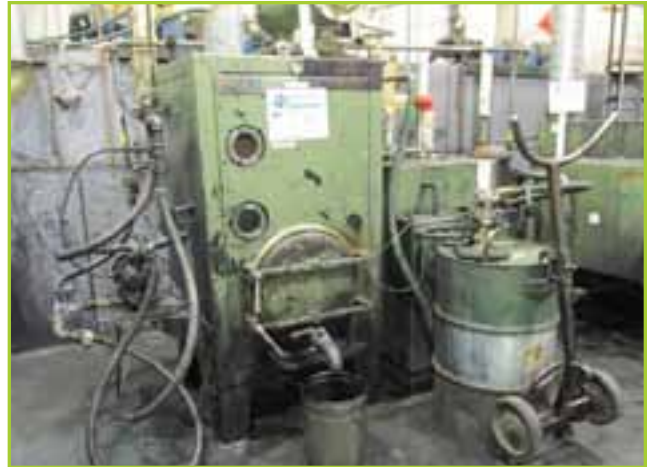
DW RENZMANN 8030 DISTILLATION UNIT , DOUBLE JACKETED. YEAR 1984
