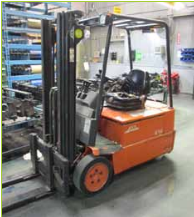
LINDEL E16-02 ELECTRIC LIFT TRUCK, #130560, 3100LB CAP., W/ CHARGER, SIDE SHIFT, SOLID TIRES, SAFETY CAGE, EXTRA BATTERY
