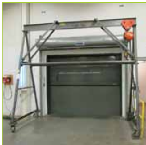
6000LB PORTABLE A-FRAME CRANE, W/ CYCLONE 3-TON CHAIN HOIST
