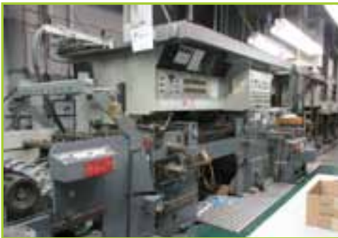
BOBST LEMANIC ROTOGRAVURE W/ IN-LINE PLA 650 ROTOGRAVURE PRINTING PRESS W/ IN-LINE PLATEN DIE CUTTER, CALIPER RANGE .010" TO .040", 12.75" TO 26" MATERIAL RANGE, LINE SPEED 180 METERS/MIN (590 FT/MIN), MAX ROLL OD 72", CORE ID 12", 10-STATIONS, 2-REVERSIBLE STATIONS, ELECTROSTATIC STATIONS; 1,2,3,4,5,6,7,8,9 , CYLINDER REPEAT RANGE 17.8" TO 25.6", 144" ELECTRIC OVEN, REGISTER CAP P/P ± 008", P/C AND P/E ± .020", ROTARY P/E ± .020", (REGISTRON S3000) TURRET ROLLSTAND, ROTARY EMBOSsing, BUTT SPLICER, 650 SPARE PARTS, 650 ROLLS, 650 INK POTS & PARTS, Q100M VISION SCANNER. YEAR 1977
