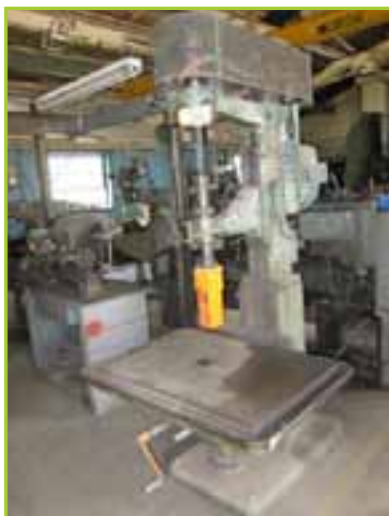
DRILL PRESS MODEL# 3B15 WITH 2HP MOTOR DRIVE, 37"X26" WORK TABLE
