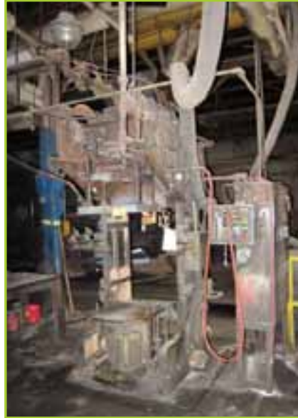
COLD BOX CORE / MOLDING MACHINE MODEL# CB-15-GF
