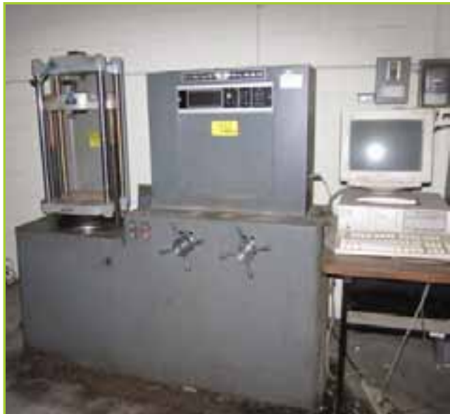
TENSILE TESTER WITH MDL.290 PLC CONTROLS, HEWLETT PACKARD PRINTER & EXTENIOMETER
