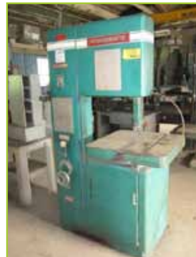
POWERMATIC BANDSAW MODEL# 87 WITH 24"X24" WORK TABLE, BLADE WELDING & GRINDING ATTACHMENT
