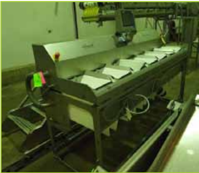
MAREL TARGET BATCHER, MODEL TBL-3000, 7 BUCKETS
