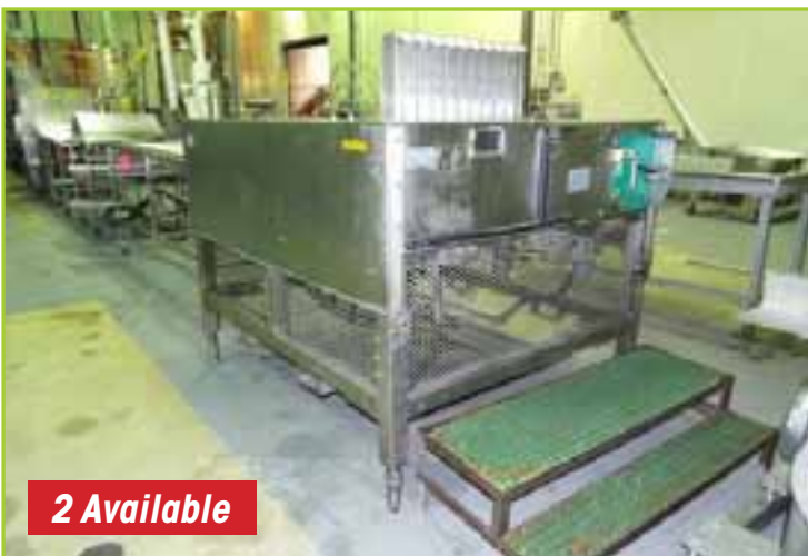
ROSS SLICER MODEL 990B, HYDROLIC MOTOR, 30 IN. WIDE BELT
