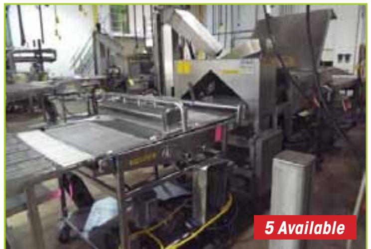
STAIN BREADER/BATTER MACHINE WITH HYDROLIC MOTORS AND BREADER RECLAIM/FEEDER, 40 IN. X 12 FT., COMPRESSOR ROLLER
