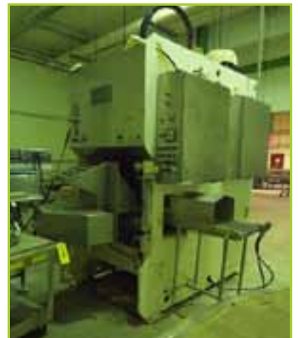
PEARSE EQUIPMENT BLOCK PRESS MODEL: BSP-55-3 WITH DIES AND INFEED CONVEYOR
