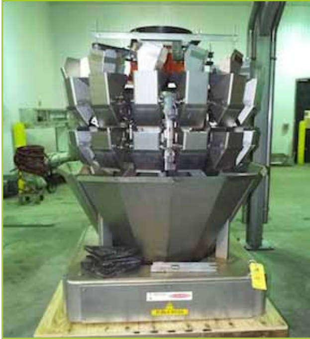
ISHIDA RODARY SCALE WITH 14 BUCKETS MDCCW-M-214W-S/30-WP, S/N 45693, JOB# 02/12425, 208-240 V, 7.4 A, 60 HZ
