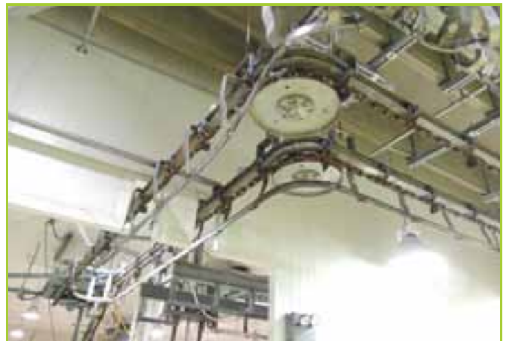
APPROXIMATELY 450' MEAT RAIL SYSTEM, WITH INCLINE, SWITCHES, DRIVE CHAIN, LOWERATOR AND DRIVES
