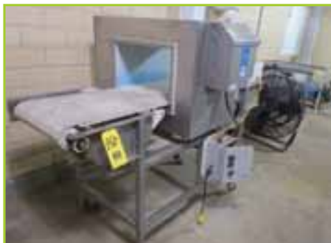
LOMA IQ2 METAL DETECTOR, WITH CONVEYOR AND 19 1/2" X 12" APERTURE
