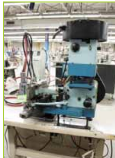
JUKI MB373 Z032 MITCHELL BUTTON ROBOT. TSS STAND WITH ELECTRIC BOX AND FOOT PEDAL
