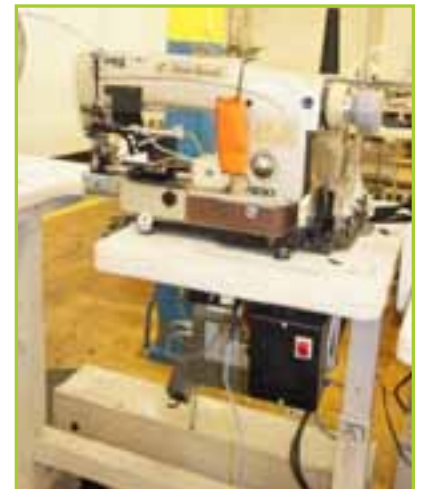
UNION SPECIAL 63900W OVER ARM HEMMER, TSS STAND WITH ELECTRIC BOX AND FOOT PEDAL. NEEDLE STOP
