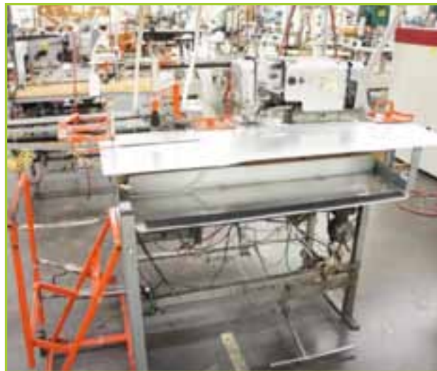
DURKOPP 556-1101/E21 TACKER, SHIRT FRONT BUTTON HOLE WITH DEAN HUNT STACKER. ADJUSTABLE SIZE BUTTON HOLES. 3/8" TO 2"
