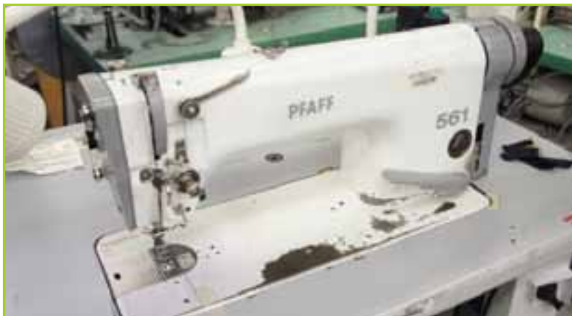
PFAFF 561-900/99 SINGLE NEEDLE LOCKSTITCH, NEEDLE FEED WHITE & TAN. (2)EFKA AC MOTOR & (1) EFKA PROGRAMMABLE DC MOTOR. NEEDLE STOP. FOOT LIFT. TRIMMER. TREAD WIPER
