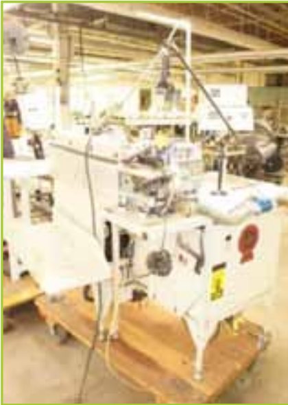
ATANTA SLEEVE HEMMER, KNIT EQUIPPED WITH PEGASUS MDL E256-1303 THREAD SINGLE NEEDLE SERGER
