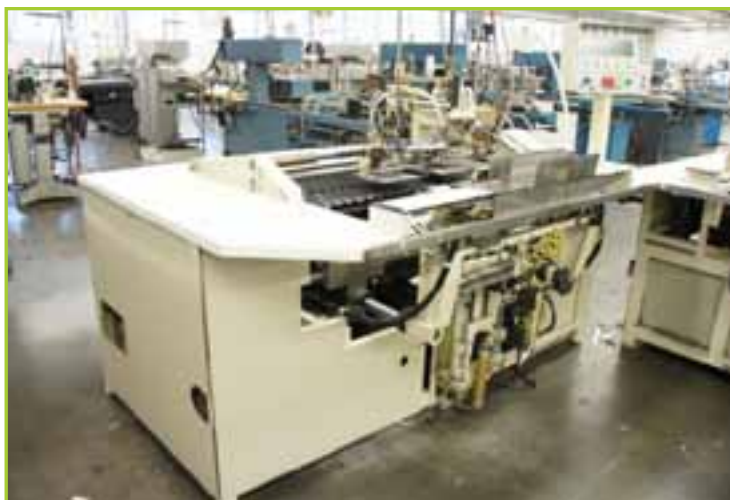
NECCHI KUAN 2684 THREAD CUTTER. NECCHI MDL 885-190 HEAD COLLAR, BAND SANDWICH PROGRAMMABLE STITCHER
