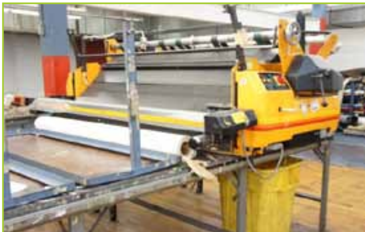
GGT NIEBUHR MA-100-MC-180-L CLOTH SPREADER, LEFT HAND MAX LOADING WEIGHT 100 KG. 220/3/60 ELECTRICS. 1998
