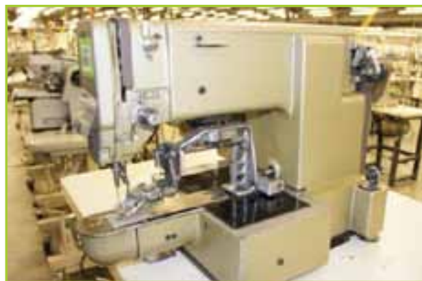
MITSUBISHI PLK-03BTA TACKER, PROGRAMMABLE BAR TACKER, TSS STAND, ELECTRICAL BOX AND PEDAL. MAX SEWING AREA X=30MM Y=30MM
