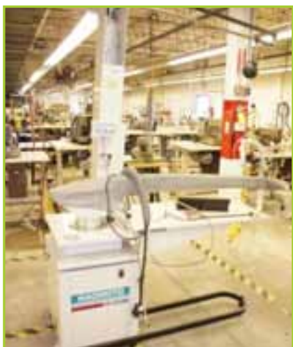
NAOMOTO J-50U HI STEAM VACUUM BOARD, SELF CONTAINED
