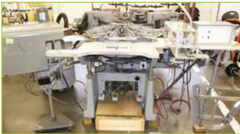
ADLER 971-800/1 RETROFITTED WITH PLC CONTROLS. UNLOADER ATTACHMENT. AND VACUUM
