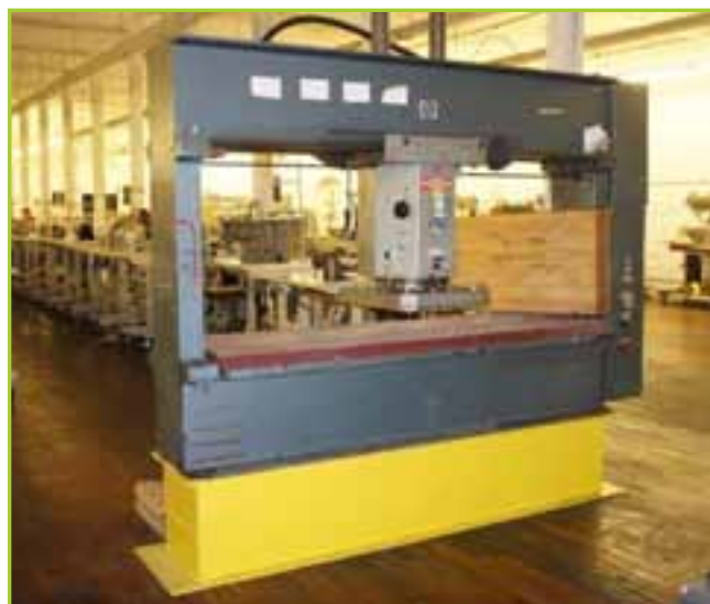
USM CLICKER, TRAVELING HEAD, HEAD SIZE 19.5" X 25.5". 81" BETWEEN UPRIGHTS
