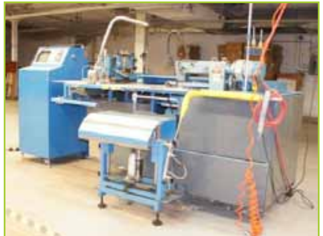
IDEAL 6864 POCKET SETTER EQUIPPED WITH TEMPLATE FOR SHIRT FRONT WITH PENCIL TUNNEL. FREE STANDING CONTROL PANEL.
