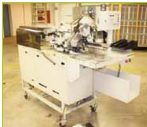
JUKI APW-232 POCKET WELT MACHINE , 10MM DOUBLE WELT LASER MARKER LIGHTS. EQUIPPED WITH JUKI LH-570 HEAD
