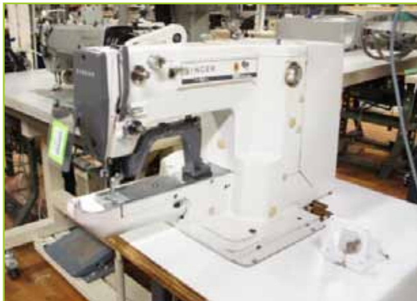
SINGER 569 U1141-28H TACKER , PROGRAMMABLE RUNNING TACK, ELECTRONIC MOTOR
