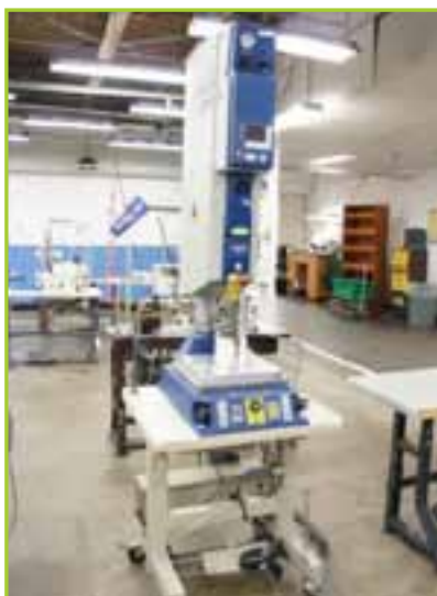
BANSON 2000 IW ULTRASONIC WELDER 20:1.1 MOUNTED ON TSS STAND, ELECTRIC BOX, FOOT PEDAL
