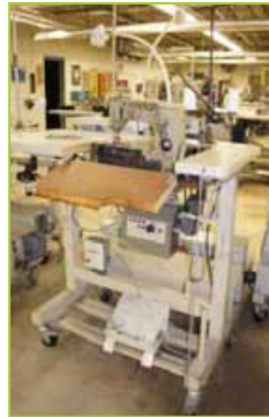
UNION SPECIAL 56300X WITH PFAFF PROGRAMMABLE DC MOTOR WITH BOX AND PEDAL
