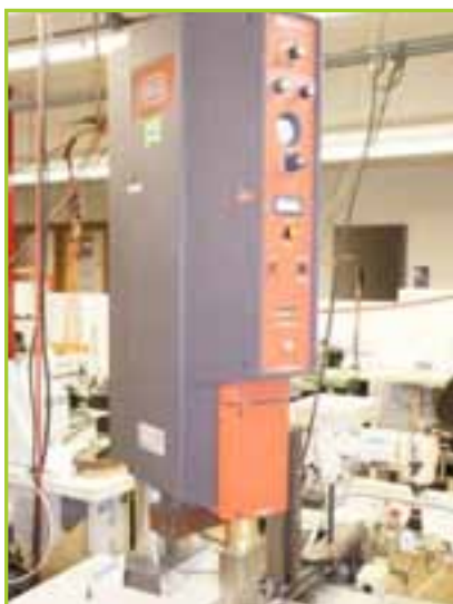
REECE (BRANSON) SERIES 72 ULTRASONIC WELDER (8400) # 47126 WITH LOADER
