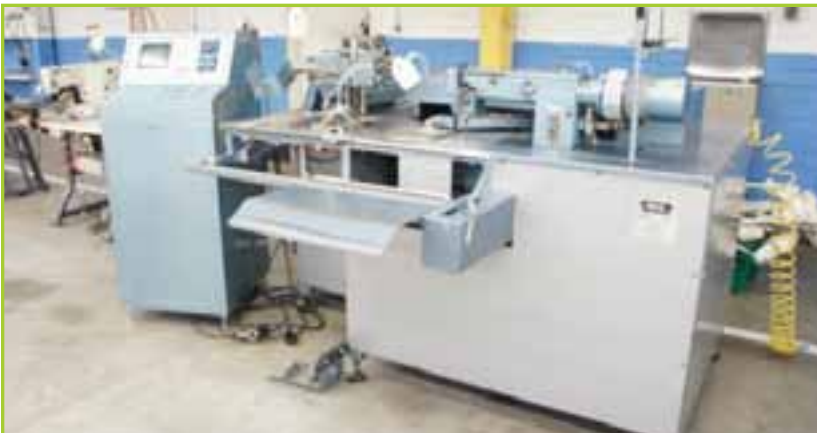
IDEAL M6052 POCKET SETTER SINGLE ROW MITER STITCHING , FREE STANDING CONTROL PANEL. CONFIGURED FOR LADIES SHIRT POCKET
