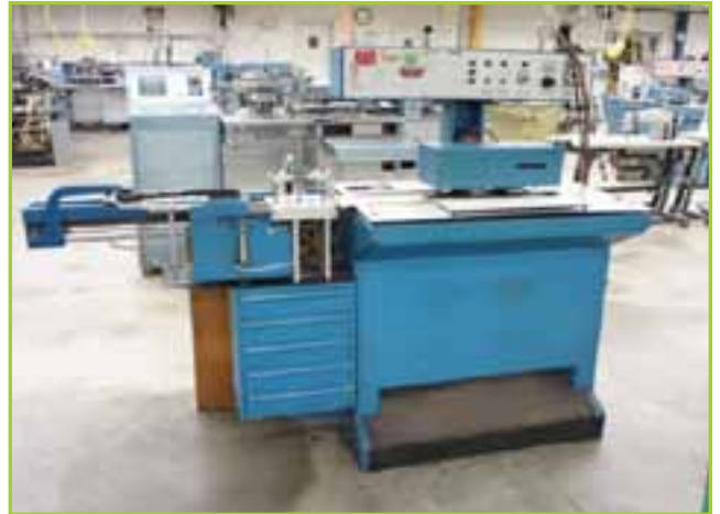
IDEAL 6020 POCKET FLAP CREASER WITH AFTER PRESS AND STACKER
