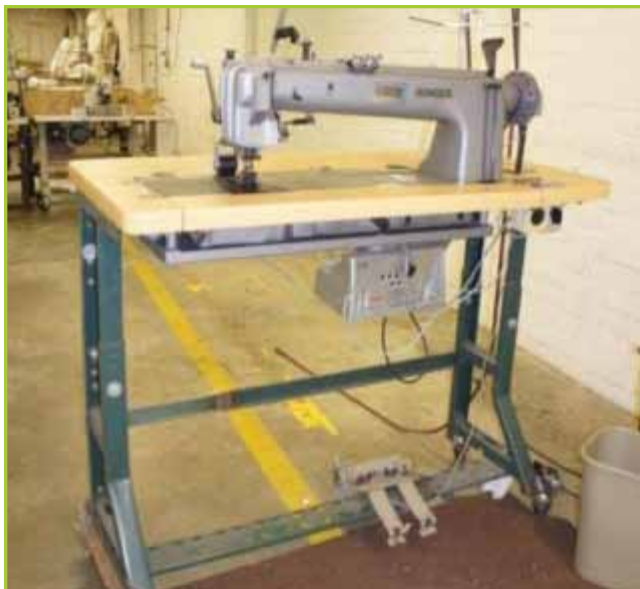
SINGER 320X2700 PFAFF PROGRAMMABLE DC MOTOR AND PANEL, SPEED CONTROL. NEEDLE POSITIONER. WALKING FOOT AND PULLER.
