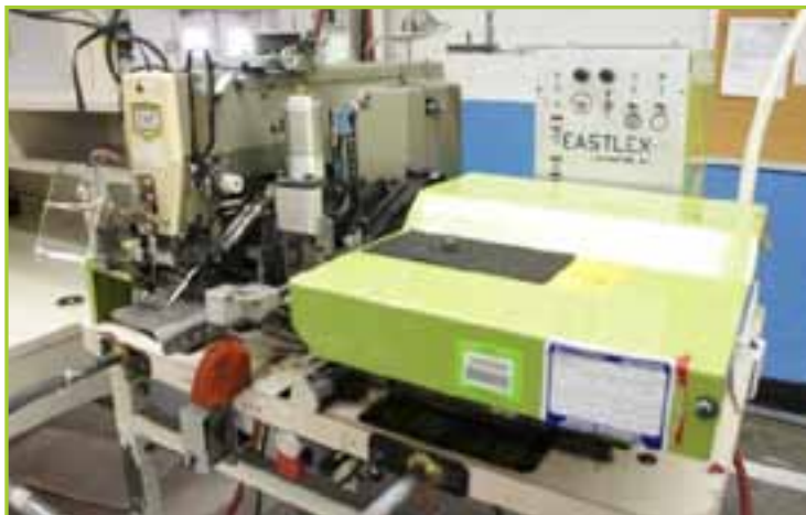
EAST LEX 7400 EQUIPPED BELT LOOP TACKER MACHINE, WITH JUKI MDL LK-1852, 110 VOLT MOTOR
