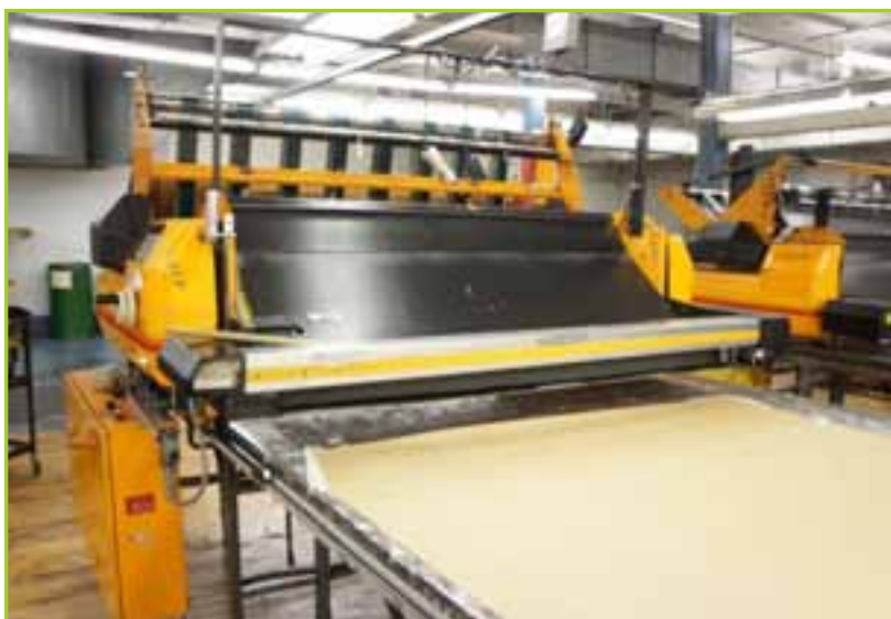
GGT NIEBUHR 5300-076-1012 CLOTH SPREADER, RIGHT HAND MAX LOADING WEIGHT 100 KG. 220/3/60 ELECTRICS. 1998
