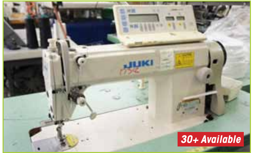
JUKI DLN-5410N-7 WB H JUKI PROGRAMMABLE DC MOTOR AND PANEL. NEEDLE STOP. TRIMMER.
