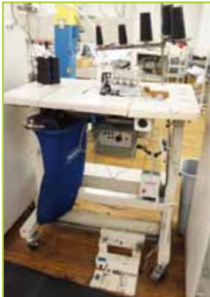
JUKI MOJ-2516N CLASS FF6-600 E QUICK DC MOTOR & PANEL. THREAD CHAIN CUTTER. TSS STAND & ELECTRIC BOX
