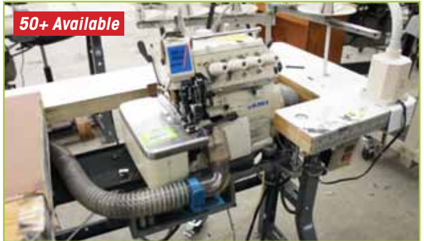
JUKI MOJ-3916 CLASS FF6-700 SERGER SAFETY STITCH 5 THREAD 2 NEEDLE QUICK DC PROGRAMMABLE MOTOR AND PANEL. TEMPLEX VACUUM ATTACHMENT. THREAD CHAIN CUTTER. AIR FOOT LIFT, NEEDLE STOP
