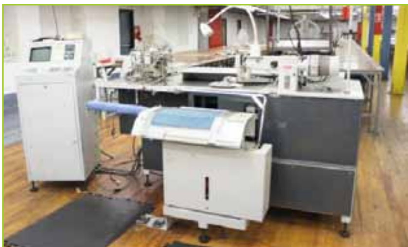
IDEAL 6864 POCKET SETTER EQUIPPED WITH TEMPLATE FOR KNIT SHIRT FRONT. FREE STANDING CONTROL PANEL
