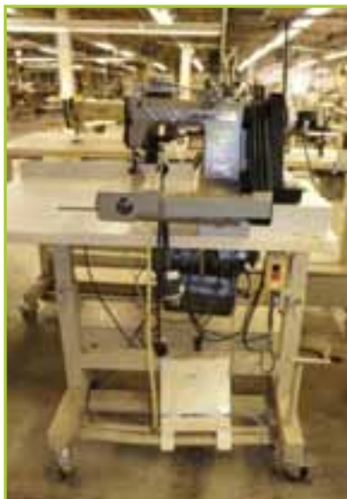
JUKI MS-261 GAUGE F RACING PULLER, TSS STAND WITH ELECTRICAL BOX/PEDAL. QUICK MOTOR & PANEL
