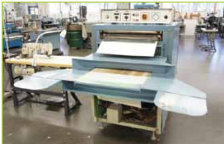
KANNEGIESSER VH600 FUSING MACHINE, 23" BELT
