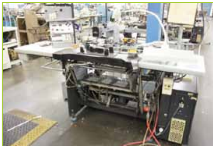
ADLER 973-S304-1 THREAD CUTTER. ADLER MDL K.1973-S204 SINGLE NEEDLE HEAD
