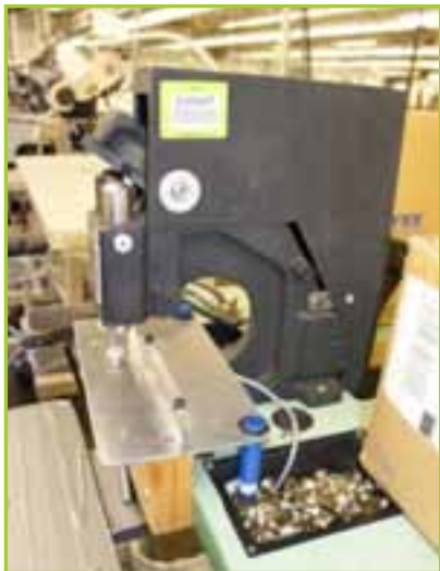
UNIVERSAL FP-2 PNEUMATIC METAL BUTTON INSTALLING PRESS
