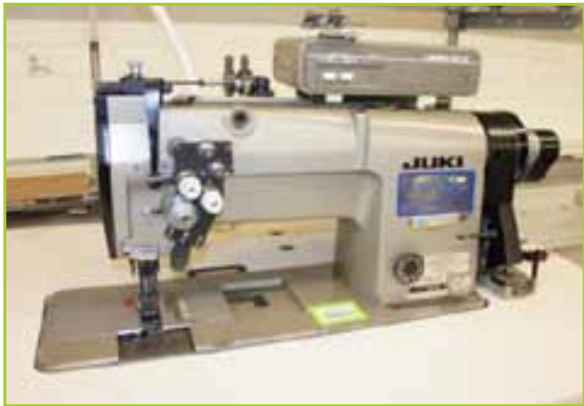
JUKI LH-1162-4 3B S GAUGE F NEEDLE STOP. TRIMMER & SPEED CONTROL. BACKTACK. TSS STAND WITH ELECTRIC BOX AND FOOT PEDAL. JUKE MOTOR
