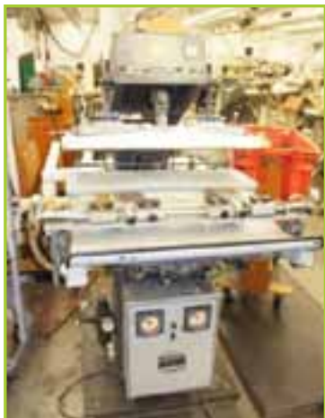
SIMPLEX 243 CONFIGURED AS CUFF PRESS, FLAT WORK 9" X 27" BED
