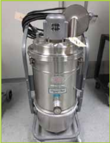
TIGER-VAC EXP1-20 DT 2009 HAZARDOUS LOCATION VACUUM , EXPLOSION & DUST IGNITION PROOF
