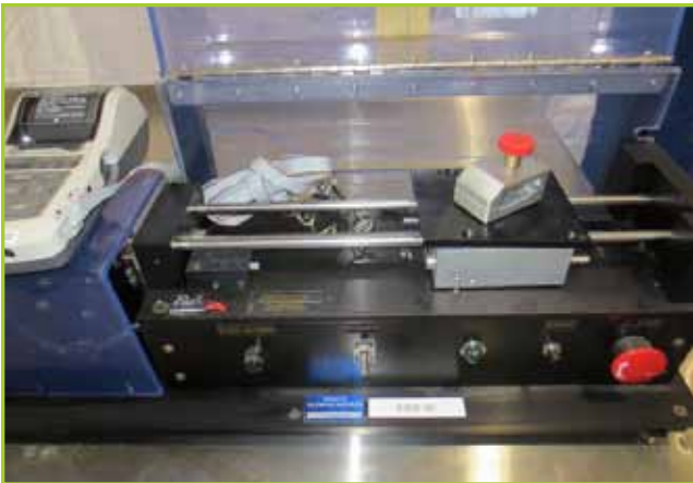
(2) VINATORU ENTERPRISE MCD HORIZONTAL SEAL STRENGTH TESTER
