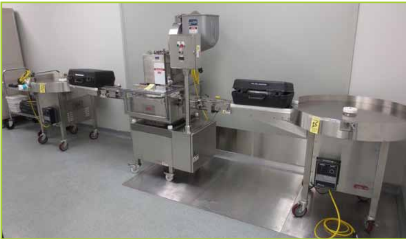
GENESIS NPW-500 WESTCAPPER 2004 AUTOMATED PHARMA CAPPER , S/N XC-31717, (2) GENESIS RU-36 ACCUMULATION TABLES, 20ML STAR WHEEL, 100ML STAR WHEEL, 10ML STAR WHEEL
