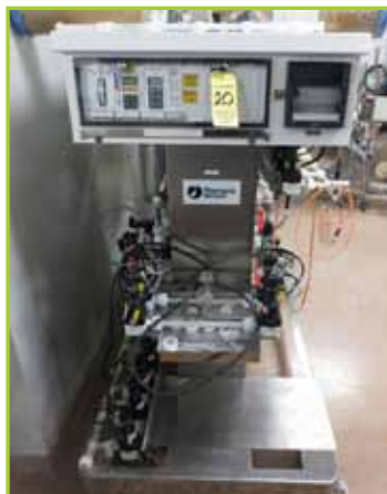
PHARMACIA BIOTECH SYSTEM 255 PURIFICATION SKID, PC, PANELS
