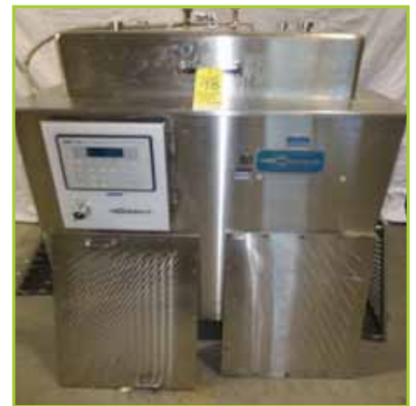
COZZOLI GW-24 VIAL/STOPPER WASHER, S/N GW24-228, MMI-240 CONTROL, (4) SPARE HOLDERS
