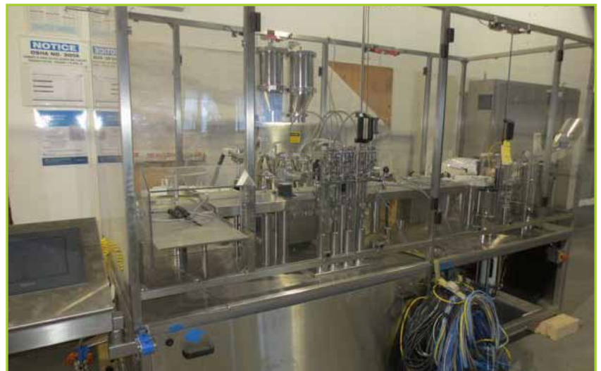
M&O PERRY CU-1013 FORM FILL AUTO FILLER , S/N P-791, POWDER & LIQUID FILLING, STOPPER INSERTION, CHECKWEIGH, 20 ML VIAL, HEPA FILTERS, (4) NEEDLE, VIAL REJECTION
