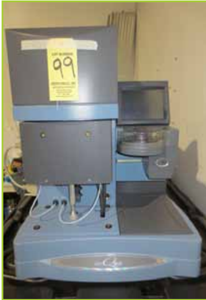
TA INSTRUMENTS TGA Q5000 THERMAL GRAVIMETRICS SYSTEM, S/N 5000-5051
