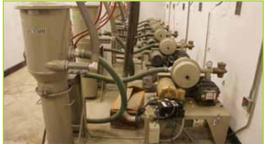
CONAIR PD5 REV TALB/0396 DUST COLLECTION VACUUM & FILTER SYSTEM
