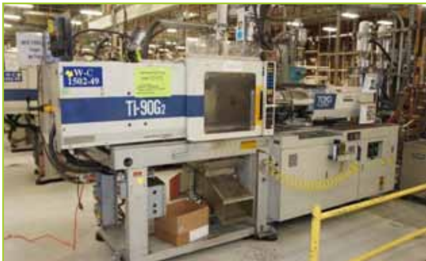
TOYO PLASTAR TI-90G2 INJECTION MOLDING PRESS; 90 USTON X 3.5 OZ SHOT. NEW 1993
