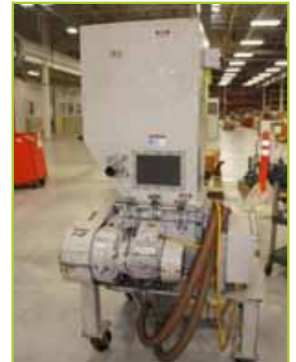
NISSUI CORP SKN-22AP GRANULATOR; 15" X 15" S CUTTER SCREENLESS
