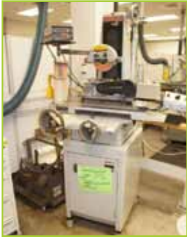
HARIG 6" X 12" MANUAL HORIZONTAL SURFACE GRINDER. WITH PAPER FILTRATION SYSTEM.
