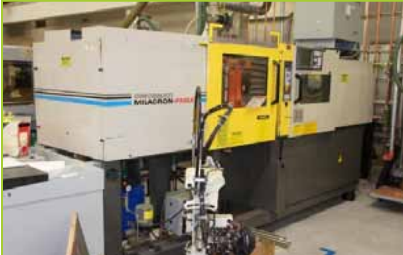
CINCINNATI MILACRON-FANUC ROBO 55R-16 55 TON TOGGLE ELECTRIC INJECTION MOLDING MACHINE. NEW 1994
