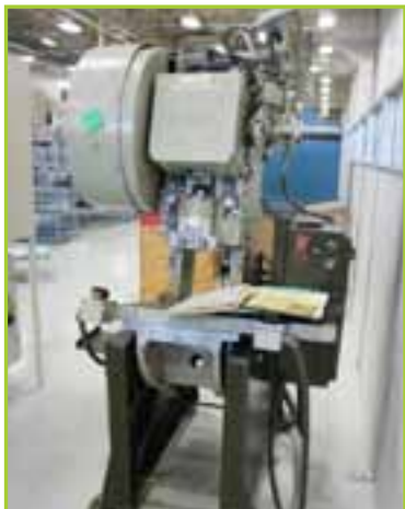
HAVIR 12 TON FLYWHEEL OBI PUNCH PRESS
