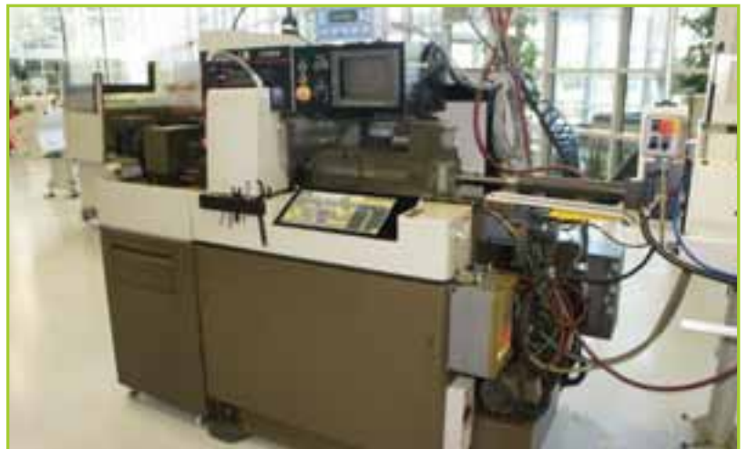
CITIZEN WATCH CO L:16/L20 16MM SWISS SCREW MACHINE, INDEX ON SUB SPINDLE
