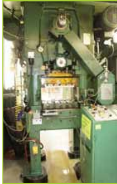
BRUDERER BSTA 30II 30T SSDC HI-SPEED METAL PRODUCTION STAMPING PRESS
