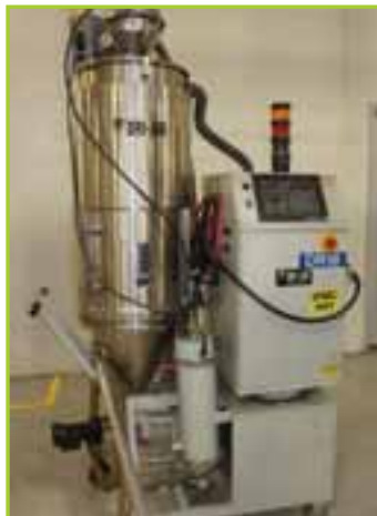
DRI-AIR HPD-4 MOLDING MACHINE 150# HOPPER DRYER LOADER
