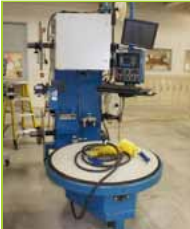
JCR AUTOMATION 5-ROW REELER W/2 CAMERA VISION INSPECTION SYSTEM
