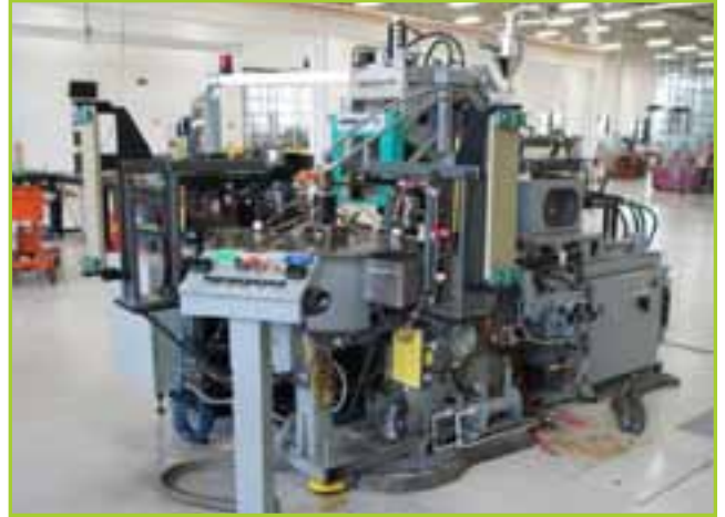
VAN DORN V1/2.30BRS NEWBURY VERTICAL MOLD CLAMPING HEAD. 4 STATION ROTARY MOLD TABLE. VAN DORN PATHFINDER 3000 CONTROLS. FREE STANDING CONTROL STATION. LIGHT SHIELD SAFETY CURTAINS. MACHINE NEW 1998
