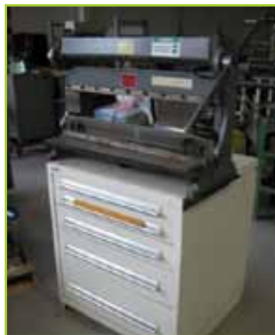
CENTRAL MACHINERY SKU T31756 30" SHEAR, PRESS BRAKE & SLIP ROLL
