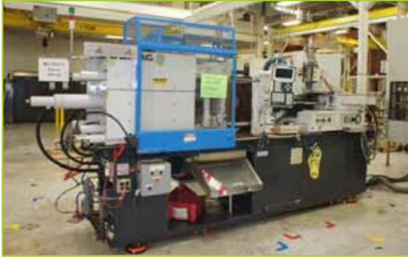
DEMAG 1000-275 INJECTION MOLDING PRESS; 100 US TON X 5.11 OZ SHOT. KNUCKLE ACTION. NEW 1994
