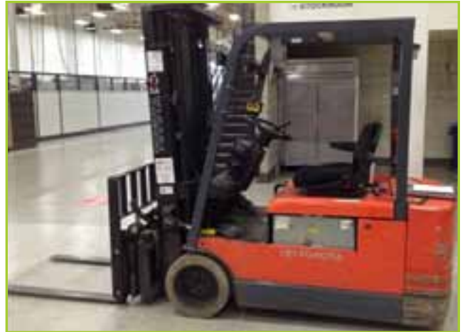
TOYOTA 5FBE20 4,000# ELECTRIC 3 WHEEL FORKLIFT
