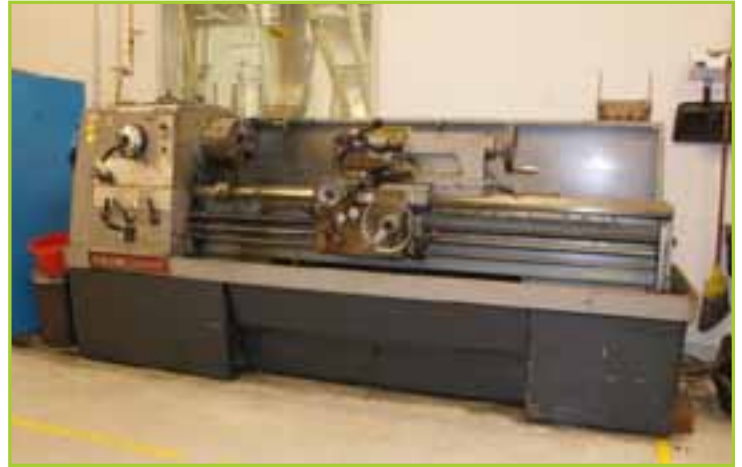
CLAUSING-COLCHESTER 7 ENGINE LATHE; 17/27" X 66" CC GAP BED. 3" SPINDLE BORE
