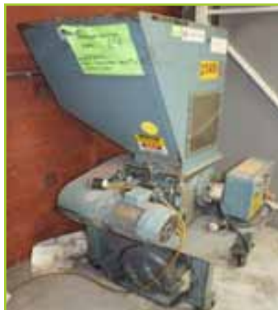
NISSUI CORP GRANULATOR; 10" X 12" S CUTTER SCREENLESS
