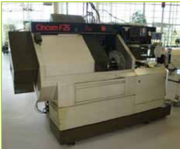
CITIZEN WATCH CO SWISS SCREW MACHINE F25 INDEXING AND LIVE TOOLING. MFG.YR. 1989
