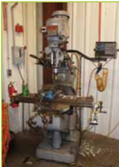
BRIDGEPORT 2HP VARI-SPEED VERTICAL MILLING MACHINE, 9" X 42" POWER TABLE
