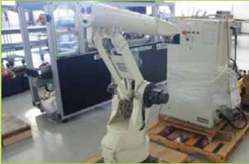
MATSUSHITA YA-TEM51 AW-005AL 5 AXIS ROBOT MANIPULATOR, FREE STANDING CONTROL BOX
