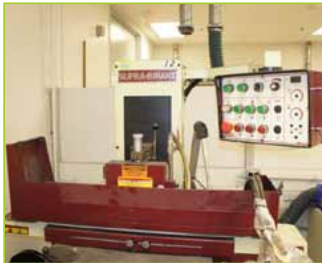
ACER SUPRA-618HII 6" X 18" HYDRAULIC HORIZONTAL SURFACE GRINDER
