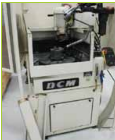
DCM ROTARY VERTICAL SURFACE GRINDER, 18" SLOTTED ROTARY TABLE
