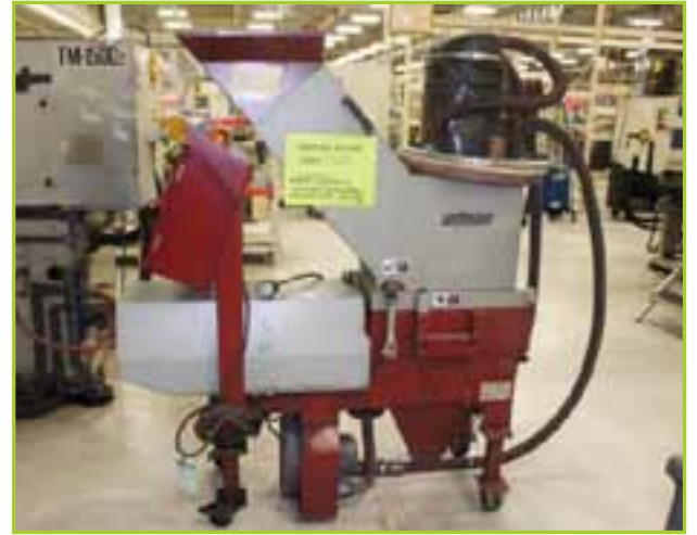
WITTMANN SJ918 GRANULATOR; 10" X 12" OPENING. 3 HP MOTOR. NEW 1991
