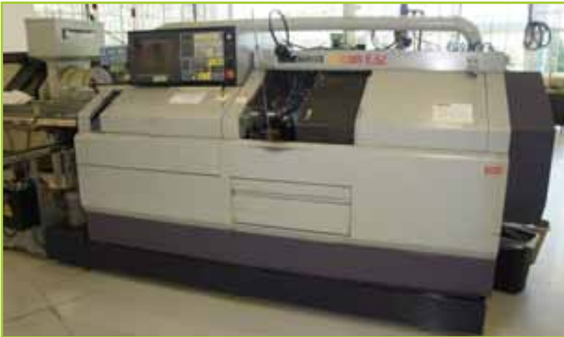
CITIZEN WATCH CO E32 SWISS SCREW MACHINE WITH SPEGO INC BAR FEED SYSTEM
