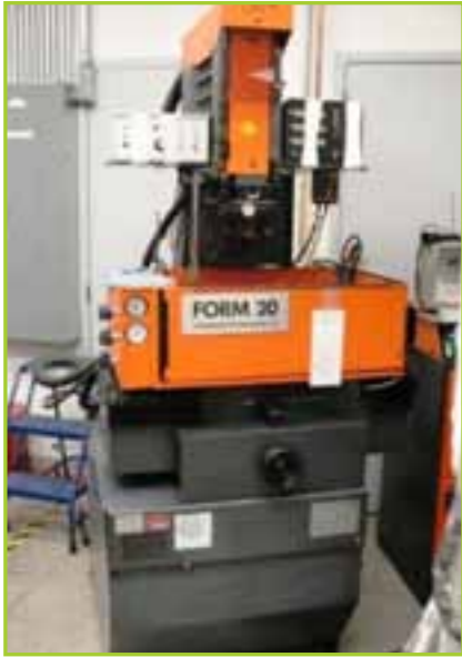
CHARMILLES TECHNOLOGIES ELECTRICAL DISCHARGE MACHINE, WIRE CUT
