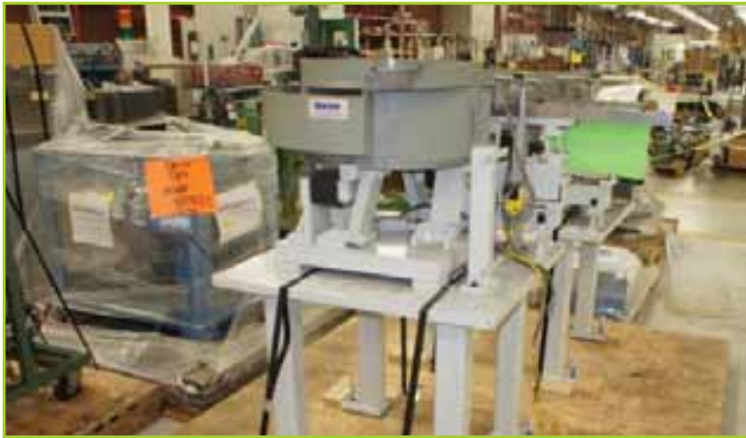
AMERICAN FEEDING SYSTEMS VIBRATORY FEED BOWLS, 24". (2) UNITS WITH COMMON CONTROL AND BOLTED TO SKID FOR SHIPMENT
