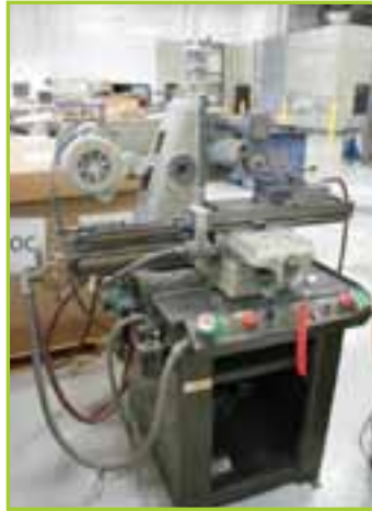
BARKER SLOTTING HORIZONTAL MILL, 4" X 16" TABLE WITH 10" FEED.
