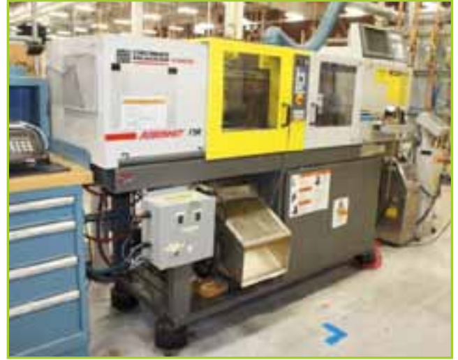
CINCINNATI MILACRON-FANUC ROBOSHOT 17R-13 17 T CNC TOGGLE ELECTRIC INJECTION MOLDING MACHINE. NEW 1999
