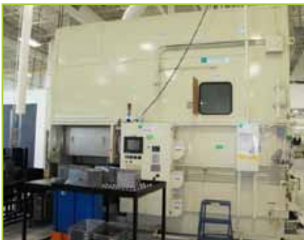
FINISHING EQUIPMENT INC RAS-30 AUTOMATIC TRAY PARTS VAPOR DEGREASER
