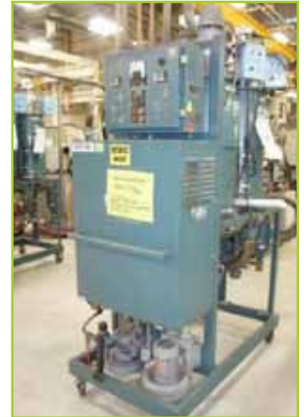
DRI-AIR ARID-X 35 PDII MATERIAL DRYER AND LOADER
