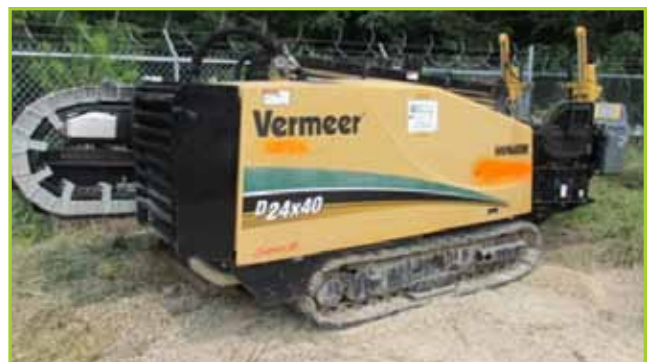
VERMEER D24X40 SERIES II HORIZONTAL DIRECTIONAL DRILLING MACHINE, CRAWLER TYPE, RUBBER TRACKS, DIESEL GAS, YEAR: 2010
