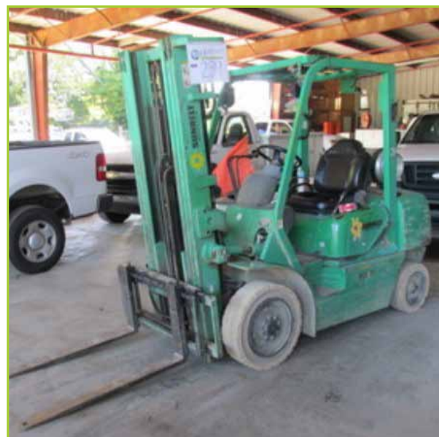
KOMATSU FG25T-14 LIFT TRUCK, LP, SIDE SHIFT, 4200 LB CAP, SIDE SHIFT
