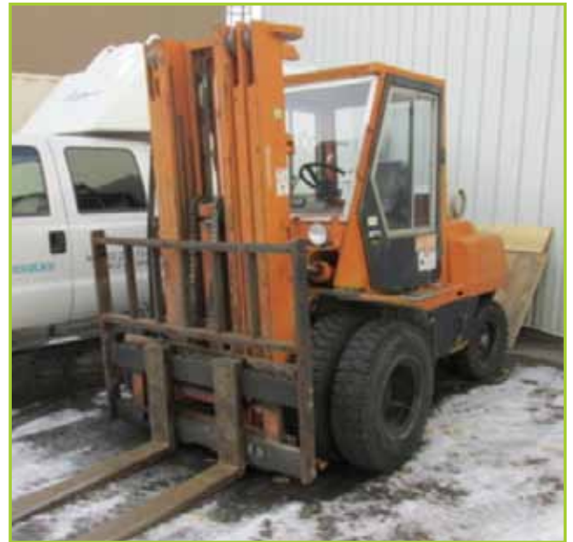
TOYOTA FORKLIFT TRUCK TOYOTA FG45 FORKLIFT TRUCK, G/LP, 8400LB CAP., SIDESHIFT, ENCLOSED CAB, DEFROST HEATER, PNEUMATIC TIRES, 8414.5 HOURS
