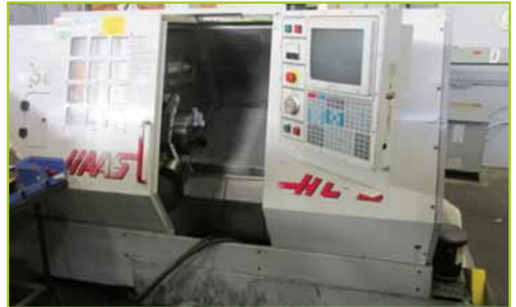
HASS CNC LATHE HAAS HL-2CNC LATHE, 2-AXIS, 2" BAR CAP, 15-HP, 3750 RPM, 10" DIA, 20" SWING, HAAS CONTROLS; YEAR: 1998
