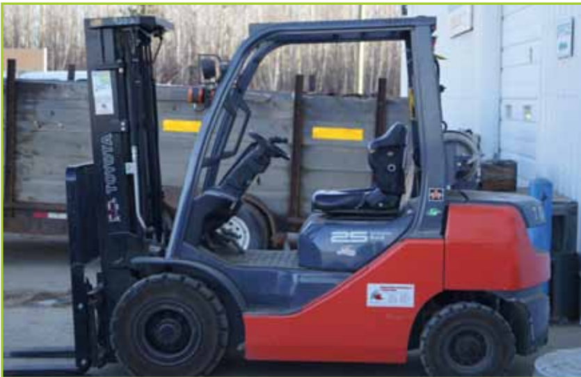
MODEL # 8FGU 25. TOYOTA LP FORKLIFT W/ SIDE SHIFTER, FSV MAST, MAX CAPACITY 3750 LBS
