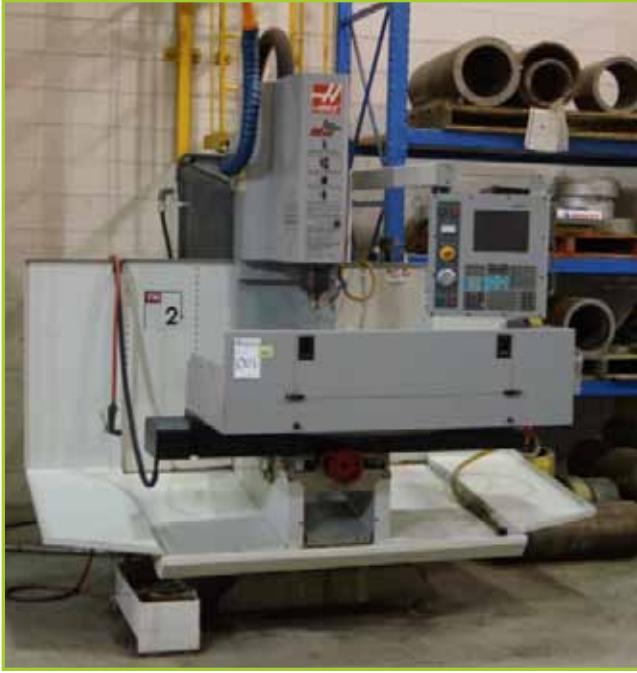
HAAS TM-2 CNC MILL. 208/240 VOLTS, 50/60 HZ, 10"X48" TABLE, DIVIDING HEAD, HAAS DIG CONTROL PAN
