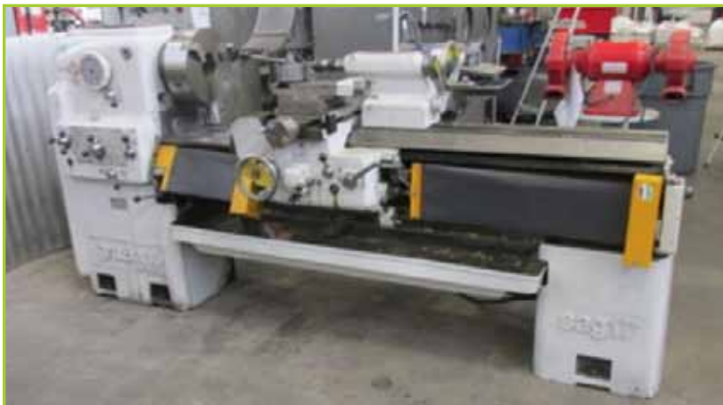
GRAZIANO ENGINE LATHE GRAZIANO SAG 17 ENGINE LATHE W/ MITUTOYO KS DIGITAL CONTROLS
