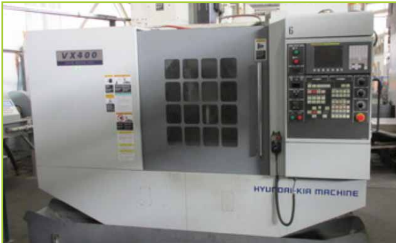
HYUNDAI-KIA VX400 CNC VERTICAL MACHINING CENTER , X,Y STROKE - 31.5" X 18.1", 1,323LBS LOAD CAP., 24-TOOL MAGAZINE, 12,000 RPM, 20-HP, FANUC SERIES 0I-MC CONTROLS, COOLANT THRU SPINDLE 230 PSI
