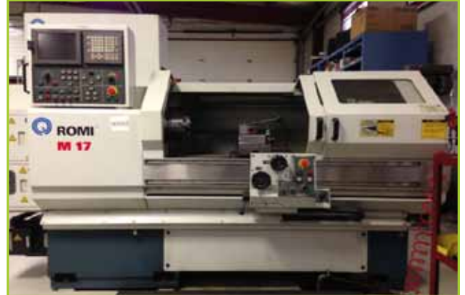
ROMI M17 CNC LATHE , 17 X 36. SWING OVER BED: 17", SPINDLE BORE: 2 1/8", BED LENGTH: 67", OPERATING SYSTEM: FANUC 21-T. WGT.: 2.9T (6400 LBS.). MANF. DATE: 2000
