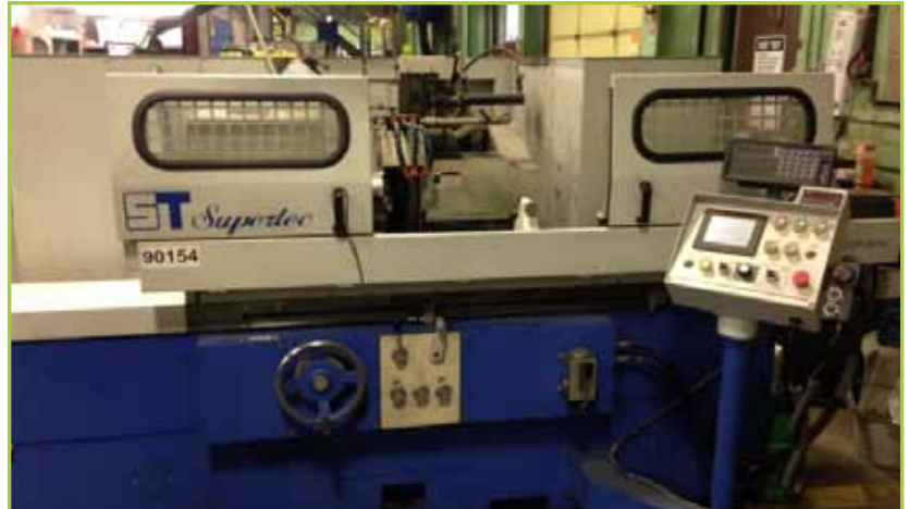
SUPERTEC G32P-100NC CNC GRINDER. SWING OVER BED: 12.598" (320MM), MAX. GRINDING LENGTH: 40" (1000MM), MAX. GRINDING OD: 12" (300MM), MAX. WORKPIECE WGT: 330 LBS. (150KG). LIKE NEW. WGT.: 4.6T (10300 LBS.)
