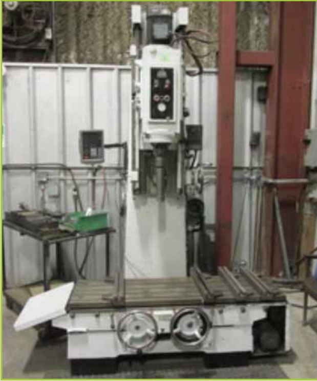
AMC VERTICAL BORING MACHINE AMC C4 VERTICAL BORING MACHINE W/ NEWELL C80 CONTROLS
