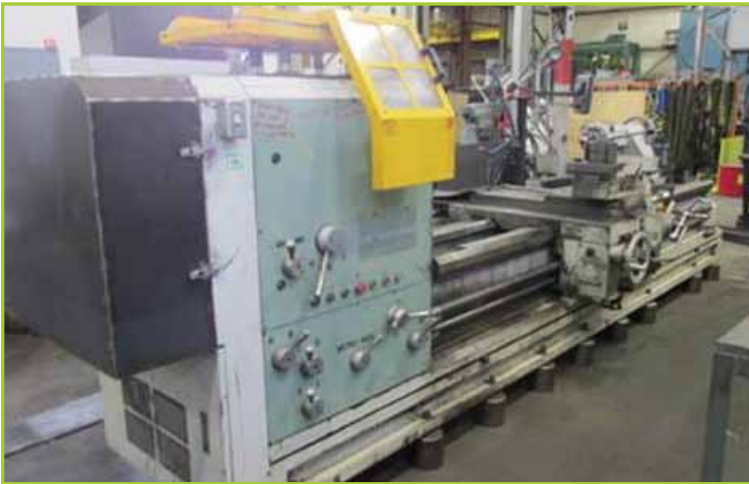
MODERN BUFFALO LATHE MODERN 35120X W/ NEWALL C80 CONTROLS, 35 X 120
