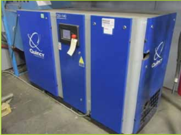
QUINCY QSI-140 ROTARY SCREW AIR COMPRESSOR, 30-HP; YEAR: 2013
