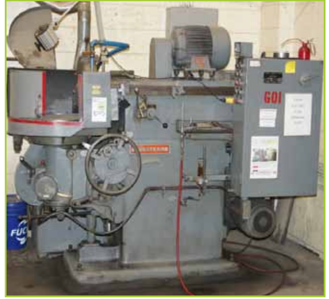
SUNDSTRAND 3RC4 ROTARY SURFACE GRINDER. 440 VOLTS, 11.75HP
