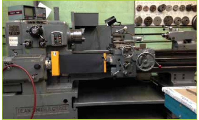
DEAN SMITH & GRACE 17 X 48 ENGINE LATHE, 17 X 48. SWING OVER BED: 16", SPINDLE BORE: 2", BED LENGTH: 72". WGT.: 2.5T (5500 LBS.). MANF. DATE: 1970
