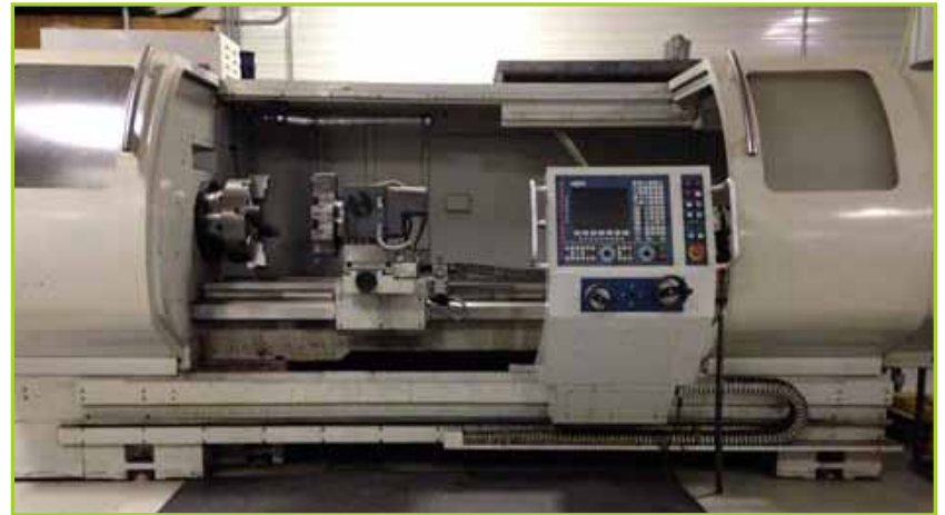
BNC 2280XL CNC LATHE, 22 X 80. SWING OVER BED: 22", SPINDLE BORE: 4", BED LENGTH: 118", OPERATING SYSTEM: FAGOR. WGT.: 4.8T (10600 LBS.). MANF. DATE: 2005
