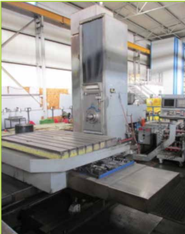
OLYMPIA CNC HORIZONTAL BORING MACHINE OLYMPIA H8060 OLYMPIA CNC HORIZONTAL BORING MACHINE W/ GE FANUC SERIES 16I-M CONTROLS, TABLE DIA 66", SWING 70", HEIGHT UNDER RAIL 62", TOOL TAPER CAT50, LIVE MILLING SPEED 2500 RPM
