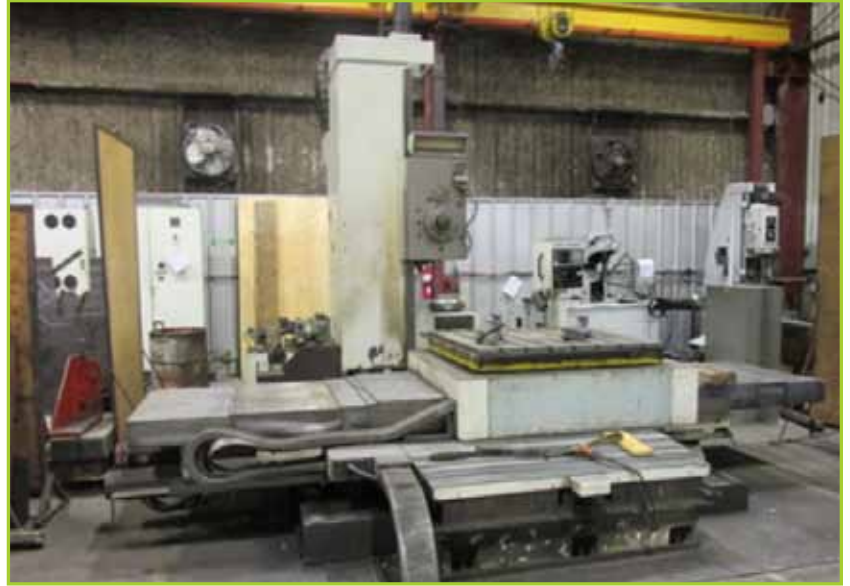
OLYMPIA CNC HORIZONTAL BORING MACHINE OLYMPIA 2B622 OLYMPIA CNC HORIZONTAL BORING MACHINE W/ GE FANUC SERIES 16I-M CONTROLS, TRAVELS X- 98", Y -63", 28" - Z, 39" -SPINDLE, 63" X 49" INDEXABLE ROTARY TABLE
