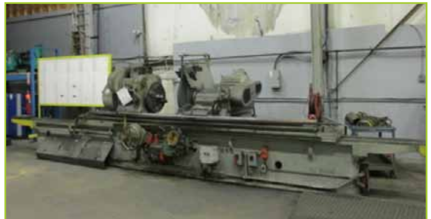
CHURCHILL DECRANKSHAFT GRINDER, 960 RPM, 40" WHEEL - 530 RPM, 40" X 180"
