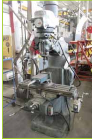
BRIDGEPORT 1-1/2 HP VERTICAL MILLING MACHINE, 9' X 36" TABLE, POWER FEED
