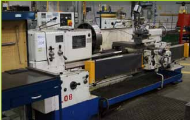
TOS TRENCIN SN63C HORIZONTAL LATHE. 220 VOLTS, 60 HZ WITH WORK BENCH
