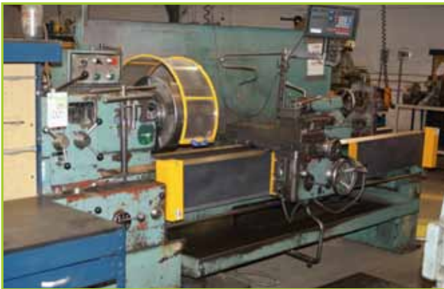
OMNITRADE SN50B HORIZONTAL LATHE. 220 VOLTS, 23 AMPS WITH WORK BENCH
