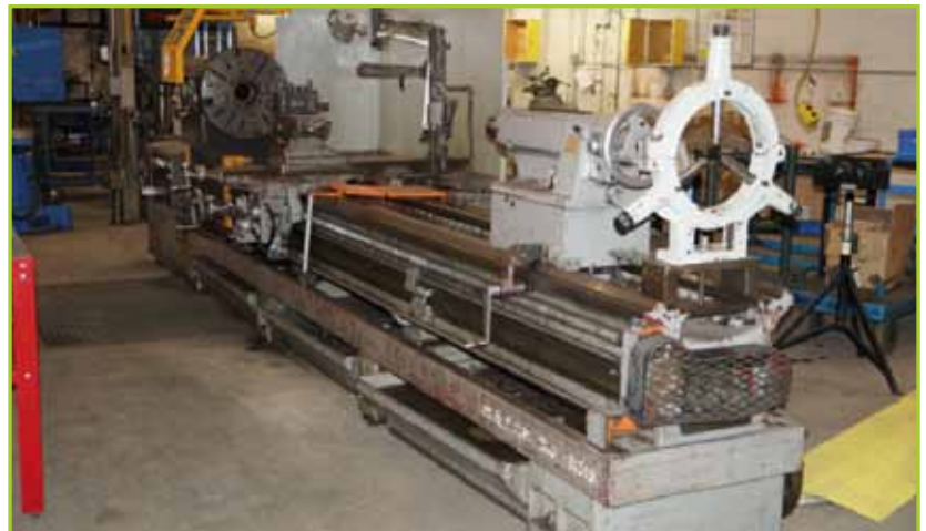
YAMAZAKI 34-160 HORIZONTAL LATHE. 34"X160", 4 1/8 SPIN BORE, NEWEL DISPLAY, 14" REST, 24X32 JAW CHUCK WITH WORK BENCH
