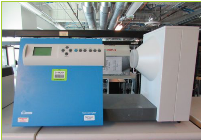
BYK-GARDNER 4725 HAZE GUARD PLUS TRANSPARENCY METER
