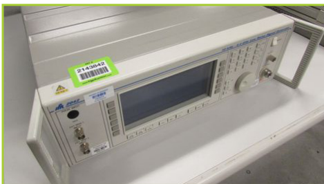
IFR SYSTEMS 2042 LOW NOISE SIGNAL GENERATOR 10 KHZ-5.4 GHZ
