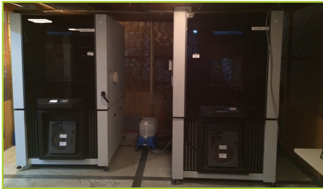
(2) THERMOTRON SE-600-10-10 TEMPERATURE/HUMIDITY CHAMBER. 40" X 33" X 27" CHAMBER, 10-95% HUMIDITY, 7-85 DEGREES CELSIUS, 230V, 60 HZ, 3 AMP, YEAR 2003
