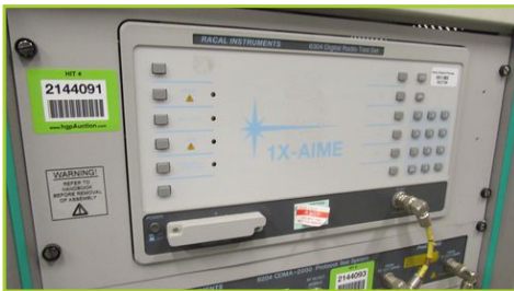
(3) RACAL 6304 DIGITAL RADIO TEST SET /BASE STATION EMULATOR UNIT INPUT- 85-130/180-264V, 45-66 HZ, 225 VA MAX
