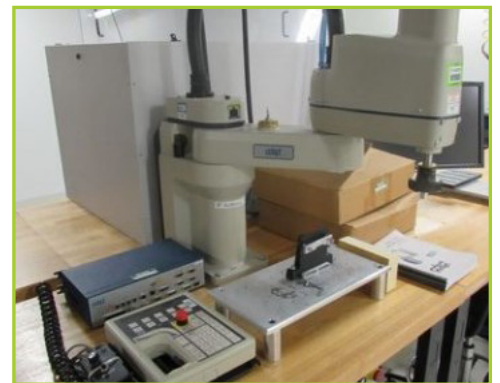
ADEPT COBRA 600 AIB COMPACT ASSEMBLY ROBOT. WITH CX SMART CONTROLLER, PENDANT, (2) ASSEMBLY CHASSIS, & COMPUTER MONITOR, YEAR 2004
