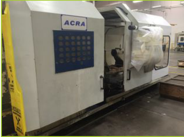
ACRA CST 42120 38"/48" X 196" LATHE , 8 STATION DUPLOMATIC TURRET, 21" SWING, SWING OVER CROSS SLIDE 27", DISTANCE BETWEEN CENTERS 120" SPINDLE SPEED: MINIMUM (RPM) 1 RPM, MAXIMUM 400 RPM, SPINDLE BORE 12", MAIN MOTOR 50/40 HP SPINDLE NOSE WITH FANUC SERIES O-T CONTROLLER AND CHIP CONVEYOR
