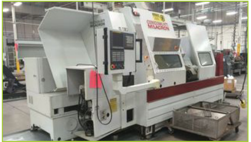
CINCINNATI MILACRON CINTURN 18U NC TURNING CENTER WITH LIVE CENTER, 8 HEAD DUAL TURRET FOR 16 TOOL POSITIONS, UPGRADED TO CNC, WITH FANUC SERIES OI-TD CONTROLLER WITH TOOLING AND CHIP CATCHERS.
