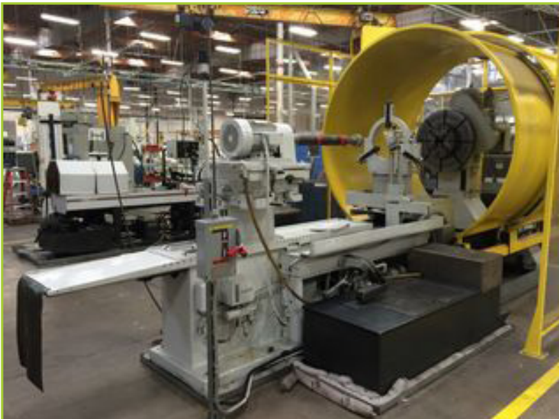
HEALD 74 64" ID GRINDING CAPABILITY, 42" GAP SWING WITH ALL SAFETY FEATURES.
