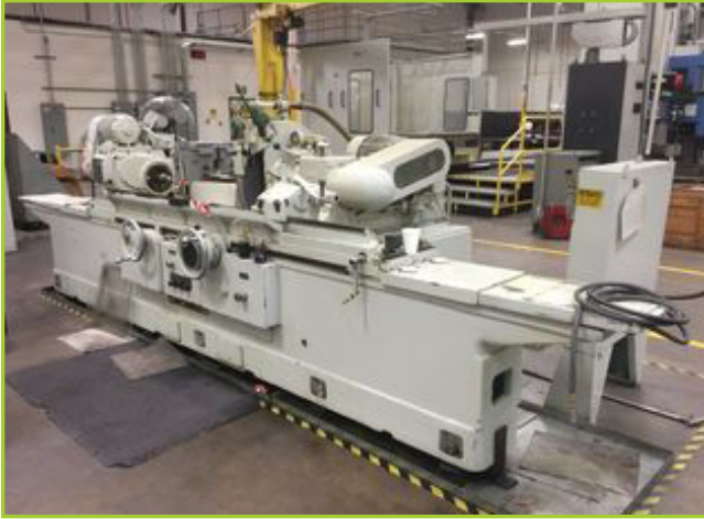
CINCINNATI MILACRON CYLINDRICAL OD GRINDER 7.5" SWING, 10" X 72" TRAVEL, 24" WHEEL.
