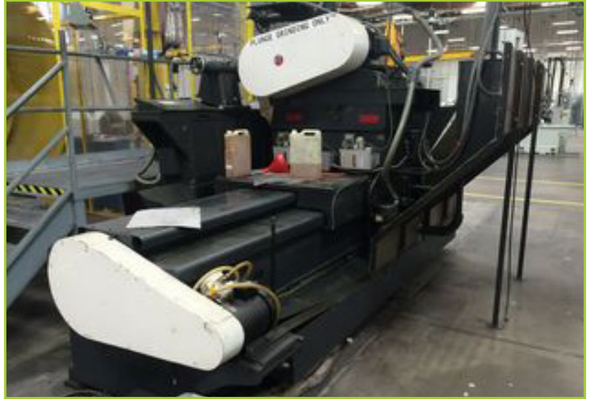
WARNER- SWASEY STRUT VARIABLE SPEED GAP BED STRUT GRINDER , MAIN SPINDLE AND SUB-SPINDLES
