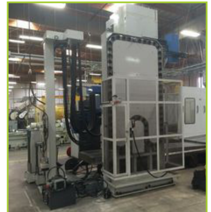
SNK NISSIN HBM BP130/3.5 5 AXIS (X/Y/Z /A/W) CNC HORIZONTAL BORING AND MILLING MACHINE , INCLUDES COGSDILL-NUNEATON ZX BOTTLE BORING HEAD, 60 TOOL, TOOL CHANGER, 86" X 63" BED, 200/220 VOLT, 3 PHASE, 60 HZ, 70 KVA (2011) WITH FANUC SERIES 311-MODEL B5 CONTROLLER.
