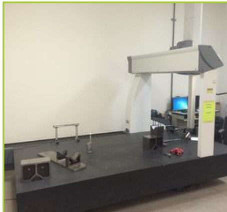
BROWN & SHARPE GLOBAL ADVANTAGE 15 22 10 (2007) 125" X 67", RENISHAW PI 200 INTERFACE FOR TP 200 SYSTEM, TESASTAR SM PROBE HEAD MODEL 03939270
