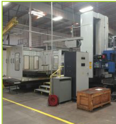
SNK NISSIN HBM BP130/3.5 5 AXIS (X/Y/Z /A/W) CNC HORIZONTAL BORING AND MILLING MACHINE , INCLUDES COGSDILL-NUNEATON ZX BOTTLE BORING HEAD, 60 TOOL, TOOL CHANGER, 86" X 63" BED, 200/220 VOLT, 3 PHASE, 60 HZ, 70 KVA (2011) WITH FANUC SERIES 311-MODEL B5 CONTROLLER.
