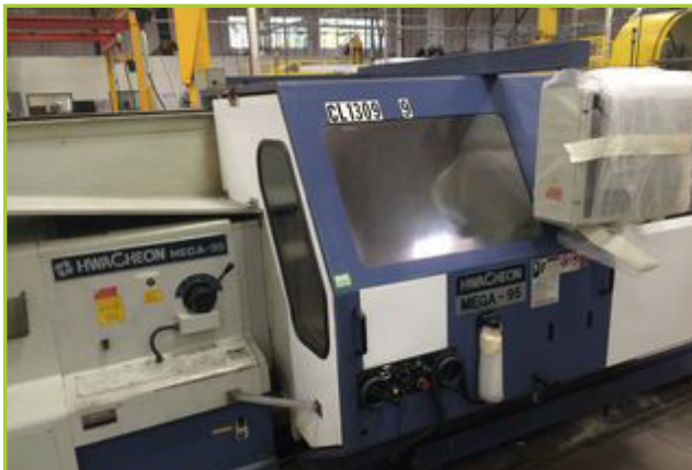
HWACHEON MEGA-95 38"/48" X 196" LATHE , 12 STATION DUPLOMATIC TURRET, 19" SWING WITH FANUC SERIES 21I-T CONTROLLER AND SMW AUTOBLOC AUTO LOCK HYDRAULIC STEADY REST, MAX SWING OVER THE BED 38" MAX SWING GAP REMOVED 48.4", MAX SWING OVER CROSS SLIDE 26.3", MAX MACHINABLE CENTER DISTANCE 196", MAIN SPINDLE MOTOR 25 HP, CHUCK SIZE 16", CROSS TRAVEL (X-AXIS) 19.09", LONGITUDINAL TRAVEL (Z-AXIS) 118", (2002) WITH CHIP CONVEYOR.
