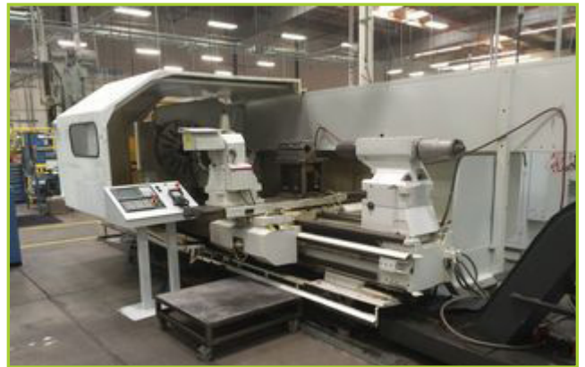
BOEHRINGER V 800 15 II LATHE, 8 STATION OD TURRET HEAD, 1 STATION ID BORING BAR STAND, 26" SWING, 380 VOLT, 3 PHASE, 60 HZ WITH MAYFRAN CHIP CONVEYOR S/N 790712-1 AND UPGRADED FANUC SERIES OI-TD CONTROLLER.
