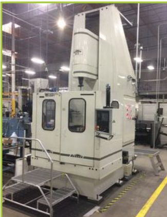
SUNNEN SV-324HT2C1E VERTICAL HONING MACHINE 40" STROKE, 460 VOLT, 3 PHASE, 60 HZ, WITH SUNNEN E615 CONTROLLER.
