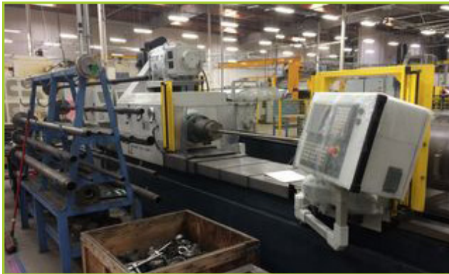
LAKER-CRAVEN 100 DEEP HOLE BORING MACHINE WITH FANUC POWER MATE CONTROLLER, STEADY REST, 110" DRILL LENGTH, KOOLANT KOOLERS HCV 10,000 2PR-NF-2FILT CHILLER, 3000 GAL. SECONDARY CONTAINMENT TANK, MAGNETIC FILTER, CHIP CONVEYOR, SAFETY FENCE, LIGHT CURTAINS AND ALL RELATED TOOLING.
