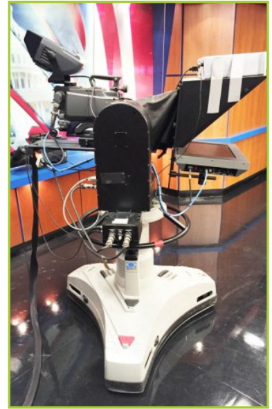
(4) VINTEN 14 ROBOTIC STUDIO SYSTEM: VINTEN HS-2010, SONY BVP-E30WS, SONY CA-570, SONY BVF-55, FUJI A18X7.6 BDERM-M48, EPD-2CA, FUJI ERD ZOOM CONTROL, QTV 15" TELEPROMPTER, VINTEN TRIPOD W/DOLLY, VINTEN AM-CSI-200, VINTEN AM-ACS-DJP, SONY RM-B150, SONY CCU-550D
