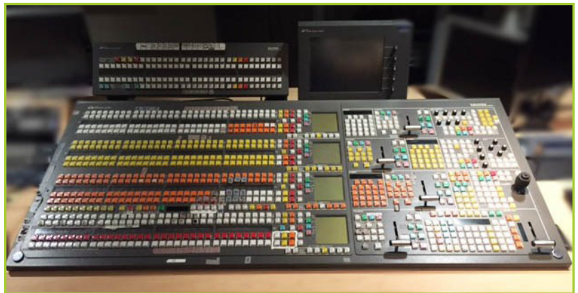
GRASS VALLEY KALYPSO 4 M/E PRODUCTION SWITCHER (M/E 1 HAS FAULTY CARD)
