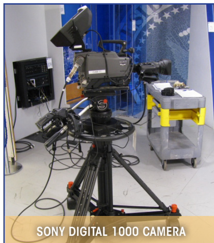
FUJINON A-14X9B LENS, SONY VIEW FINDER BFV-55 WIDE SCREEN
