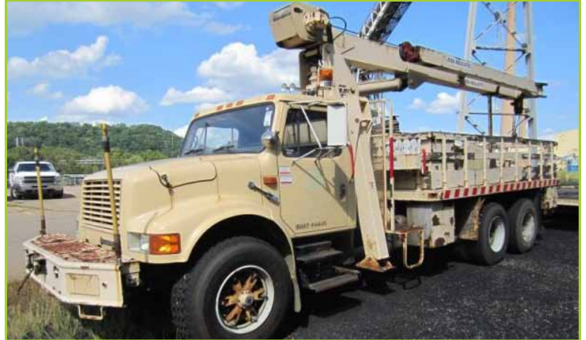
INTERNATIONAL 30FT BUCKET TRUCK. YR 1993, MODEL 1250 JBT BOOM, 18,197 MILES WITH MILLER DIALARC 250P AC/DC WELDER. VIN # 1HTSHBCTOPH524604
