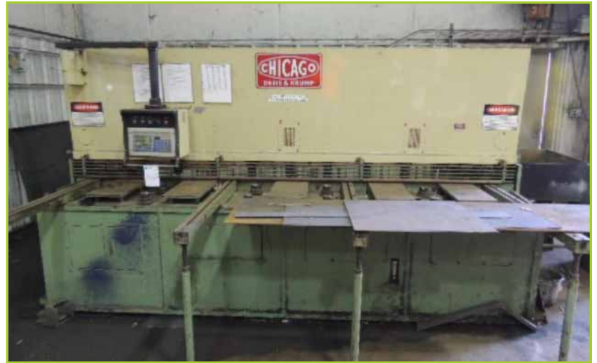
CHICAGO DREIS & KRUMP HS31130 SHEAR , ALLEN BRADLEY CONTROLS, TABLE 120" LENGTH, 1/4" STEEL, 1/8" STAINLESS, FOUR STOCK SUPPORT ARMS
