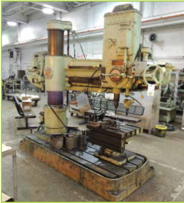
CINCINNATI BICKFORD SUPER SERVICE RADIAL DRILL , 13" COLUMN, 32" HEIGHT, 6' ARM, 575V, TILT TABLE 28"X24"
