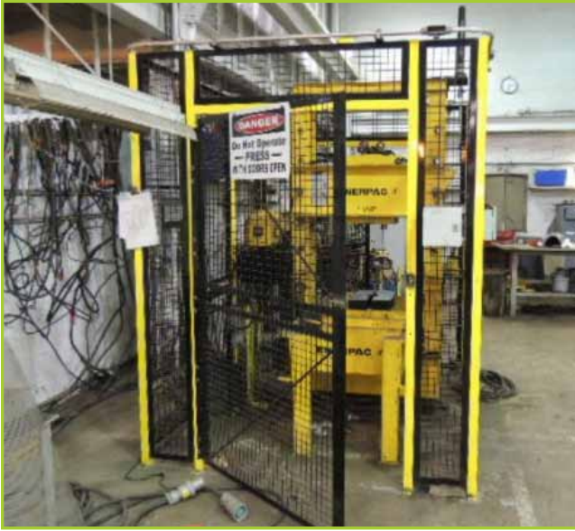
ENERPAC ZE 542056-N 100TON PRESS , MFG..2005, MAX PSI 10000 (700), ENERPAC 3HP MTR. 208-240V, WITH PROTECTIVE CAGE
