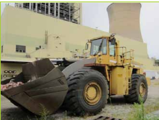
MICHIGAN L320 FRONT END LOADER. 3661 HRS, YR 1994, CUMMINS KTA19C DIESEL, 450HP
