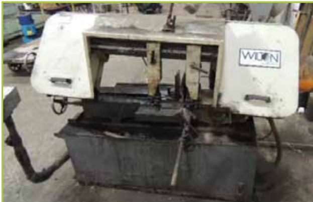
WILTON 8007060 BAND SAW , 1" BLADE X.037X156", RPM 90-370, 3HP 3PH 550V, INDUCTION MOTOR
