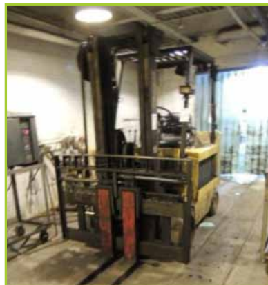
HYSTER E 100XL3S ELECTRIC FORKLIFT. 48V, CAPACITY 8700LB. LIFT HEIGHT 131.9", 72" FORKS
