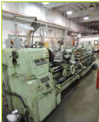
MONARCH LATHE YR. 11/1952 , 20", 26.5" SWING, 144" CENTER TO CENTER, 550V. (1) CART (1) CABINET W/TOOLING
