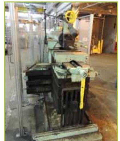
OHIO MACHINE TOOL SHAPER , P/N 1819, VISE DEEP STEEL FACED JAWS, TABLE 16"X26"
