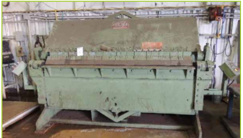
CHICAGO DREIS & KRUMP PBP 8250-6 PRESS BRAKE , POWER CLAMPING, TOP ADJUSTMENT, POWER BENDING, 96"
