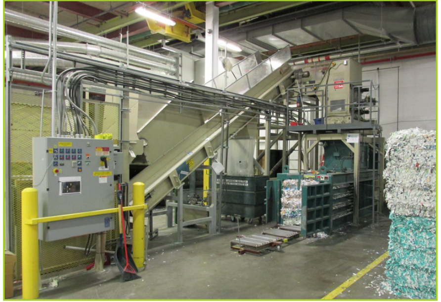
MATERIAL DISPOSAL SYSTEM, CONSISTING OF CONVEYOR/TIPPER, W/ 70 PLASTIC TOTES, SHRED-TECH SINGLE ROTOR SHREDDER, SELCO HL-12XHDM 8" CYLINDER CLOSED DOOR BAILER
