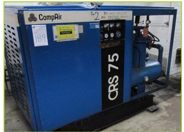
COMP AIR CRS75 COMPAIR ROTARY AIR COMPRESSOR, 75-HP
