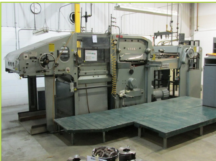
BOBST SP1080E SHEET FEED DIE CUTTER , 350 X 295 MM TO 1,080 X 780MM MATERIAL CAP., LINE SPEED 3,700 SPH, REGISTER CAP ± 0.10", W/AUTO STRIPPING, (REBUILT 1988), W/BLADES & CABINETS. YEAR 1967
