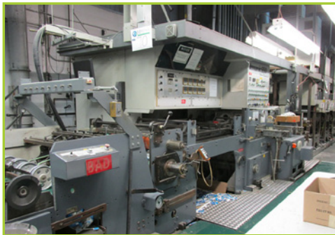
BOBST LEMANIC ROTOGRAVURE W/ IN-LINE PLA 650 ROTOGRAVURE PRINTING PRESS W/ IN-LINE PLATEN DIE CUTTER, CALIPER RANGE .010" TO .040", 12.75" TO 26" MATERIAL RANGE, LINE SPEED 180 METERS/MIN (590 FT/MIN), MAX ROLL OD 72", CORE ID 12", 10-STATIONS, 2-REVERSIBLE STATIONS, ELECTROSTATIC STATIONS; 1, 2, 3, 4, 5, 6, 7, 8, 9, CYLINDER REPEAT RANGE 17.8" TO 25.6", 144" ELECTRIC OVEN, REGISTER CAP P/P ± 008", P/C AND P/E ± .020", ROTARY P/E ± .020", (REGISTRON S3000) TURRET ROLLSTAND, ROTARY EMBOSING, BUTT SPLICER, 650 SPARE PARTS, 650 ROLLS, 650 INK POTS & PARTS, Q100M VISION SCANNER. YEAR 1977
