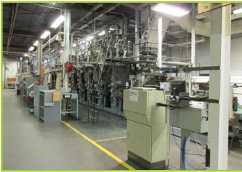
MASSON SCOTT THRISSSELL ROTOGRAVURE PRINTING PRESS W/IN-LINE ROTARY DIE CUTTER. CALIPER RANGE .010" TO .040", 14" TO 25-3/4" MATERIAL RANGE, LINE SPEED 210 METERS/MIN (689 FT/MIN), MAX ROLL OD 72", CORE ID 12", 12-STATIONS, NUMEROUS COMBINATIONS WITH TUMBAR REVERSIBLE STATIONS, ELECTROSTATIC STATIONS; 1, 3, 5, 7, 9 & 0, 2, 4, 6, 8, 19, CYLINDER REPEAT RANGE 15" TO 27", 72" ELECTRIC OVEN, REGISTER CAP. P/P ± 008", P/C AND P/E ± .020", (REGISTRON S2000), 2-TURRET ROLLSTAND, ROTARY EMBOSsing, BUTT SPLICER, CARTON ALTERNATOR MST SPARE PARTS. YEAR 1967
